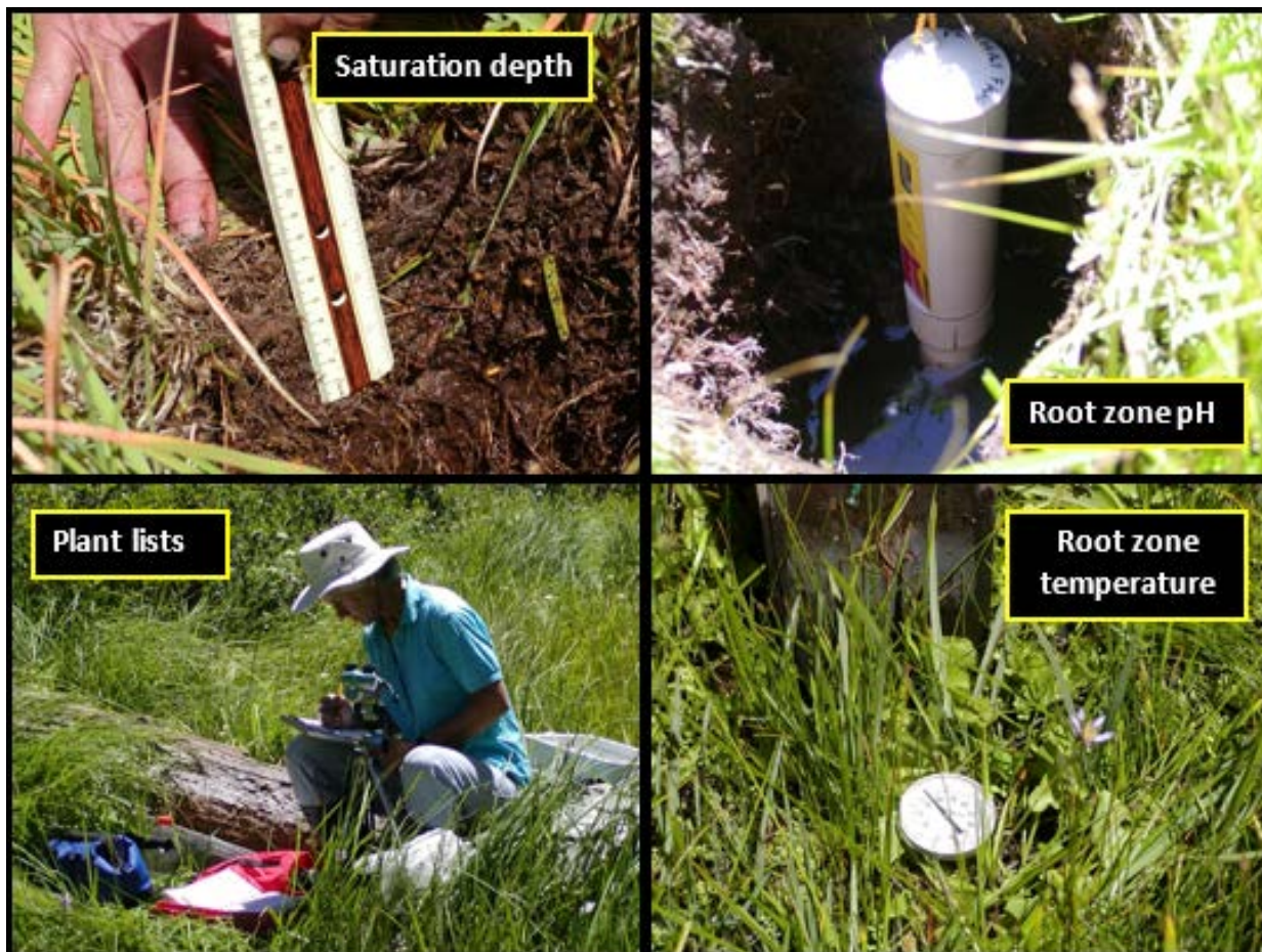
Figure 5. Survey methodology. A sample hole was dug and allowed to fill with water typical of the rooting zone of the fen plants. Temperature of the rooting zone and pH of that water were measured, representing conditions at approximately 15 to 20 cm depth. As many plants as possible were identified in the fen opening. Peat depth was measured, to at least 40 cm depth.
