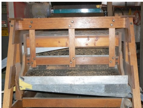
Pre-cleaning grass seed with the two-screen scalper (Alaska Plant Materials Center photo).
