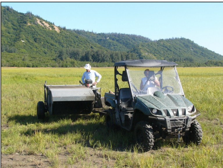
Seed stripper set-up collecting Lyngbye's sedge ( Carex lyngbyei ) on the Fox River Flats near Homer, Alaska.
