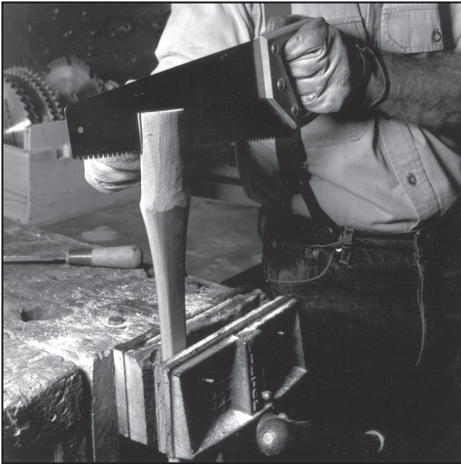
Figure 51—Since you've cut off the excess portion of the new handle, the wedge kerf slot is too shallow and must be deepened. Use a hand saw to cut the saw kerf deeper for the wood wedge. The cut should be approximately two-thirds the depth of the ax eye.
