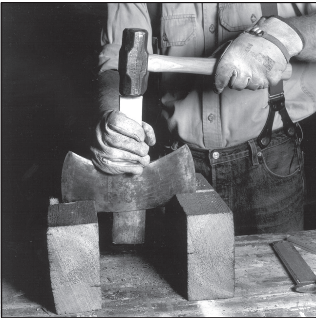
Figure 44 —Block up the ax head upside down. Drive the drift down through the bottom of the ax eye toward the top of the ax eye. The ax eye is tapered larger on the top to facilitate wedging the handle tight. This taper requires the old handle piece to be driven out the top of the ax eye.
