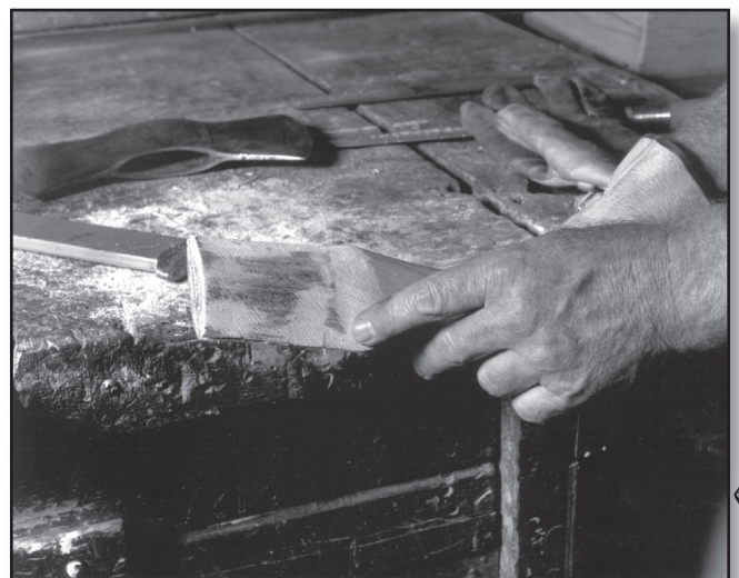
Figure 50—Drive the handle out again using a drift, and take one final rasp for a good tight fit down on the shoulder. The ax head will leave marks on the high spots that need additional light rasping.
