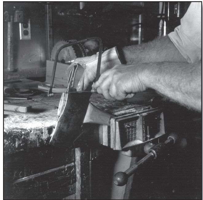
Figure 54—With a coping saw, cut the protruding handle flush with the ax head.
