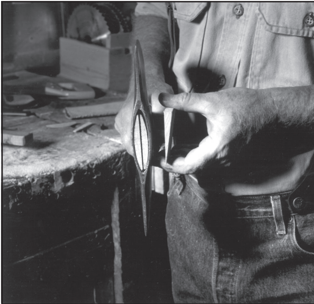
Figure 55—The fitted handle is ready for wedging. Use a correctly sized wooden wedge, usually made of well-seasoned yellow poplar or other hardwood. Avoid plastic or steel wedges.
