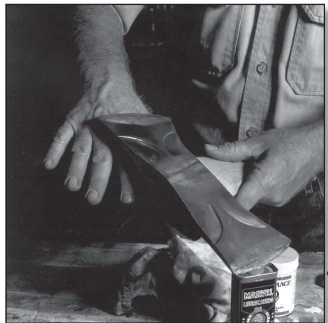
Figure 73—Shaving hair on the back of your hand is a traditional method of checking an ax's sharpness. A safer method is to place your fingernail against the edge. The edge should bite into your fingernail.
