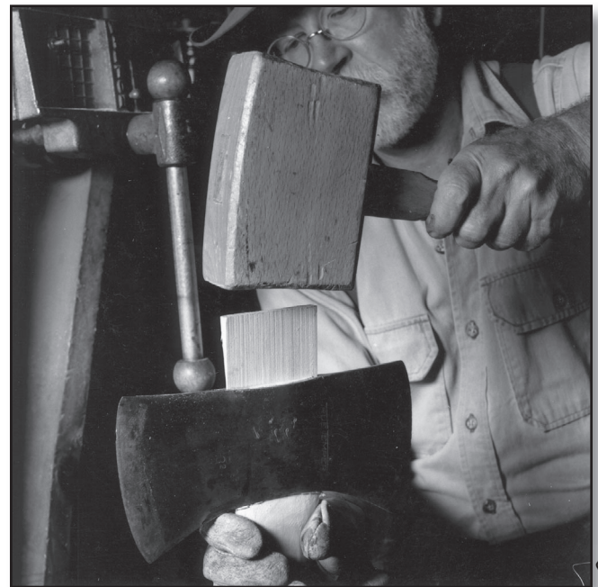
Figure 58—Insert the wooden wedge. Rest the handle bottom on something solid. Drive the wedge squarely and firmly into the kerf with a wooden carpenter's mallet. Only one-fourth to one-half inch of the wedge should protrude above the top of the handle when the wedge has been driven to the point of refusal. Use a coping saw to cut off any excess wedge.
