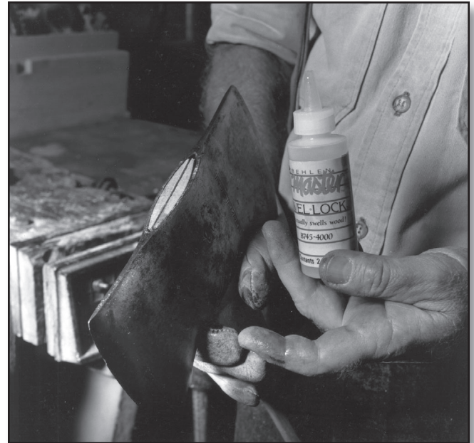
Figure 57—Before inserting the wedge in the handle, apply a coat of Swel-Lock to the inside kerf cut and the new wooden wedge. Swel-Lock is a product that swells wood. It is not a glue or an adhesive; rather, it penetrates and expands wood fibers to keep the new handle tight.
