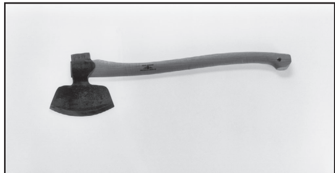
Figure 29—Modern hand-forged broad ax made by the Swedish Company, Gränsfors Bruks AB.
