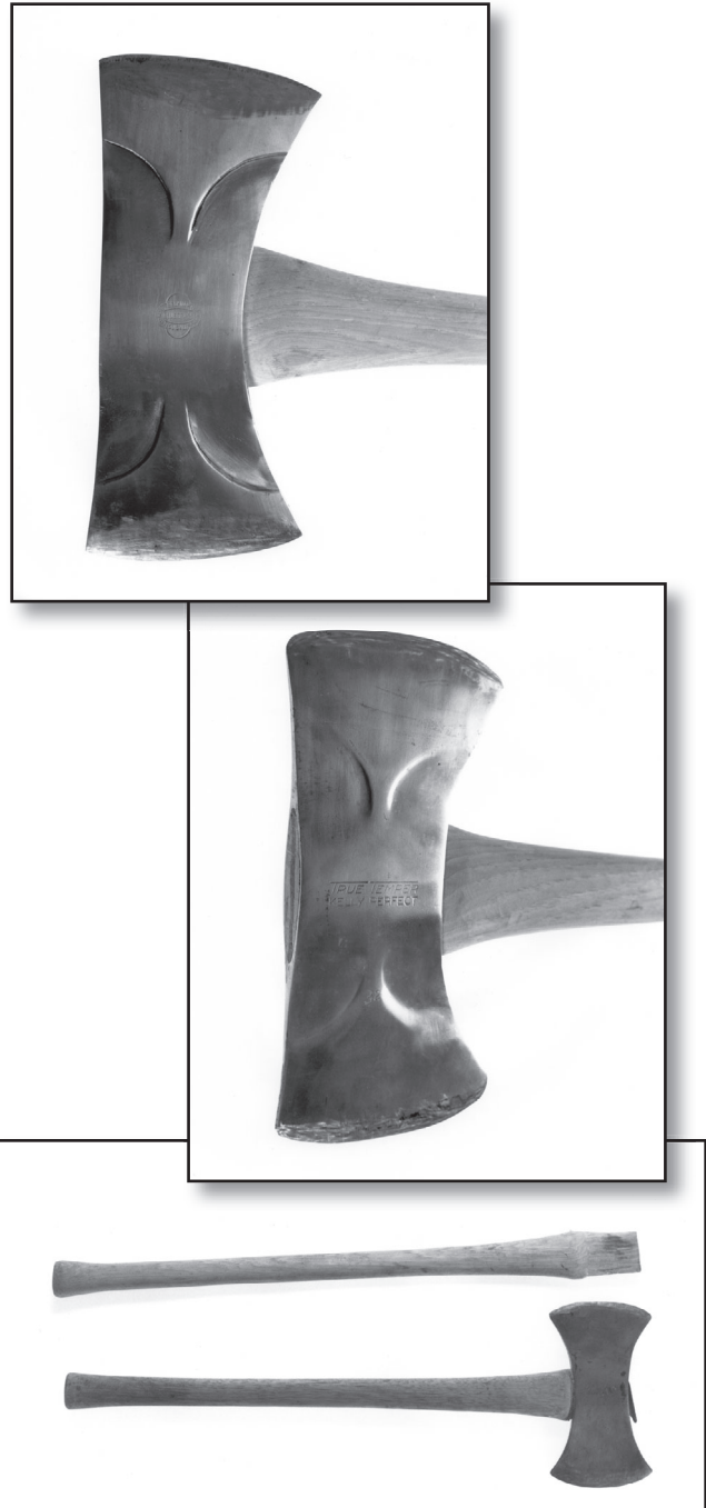
Figure 15—Three representative double-bit patterns: Bluegrass Western pattern double-bit ax (top); True Temper Kelly Perfect Michigan pattern double-bit ax (middle); and a 2 1/2 -pound reversible cruiser ax, sometimes used for ax throwing (bottom).
