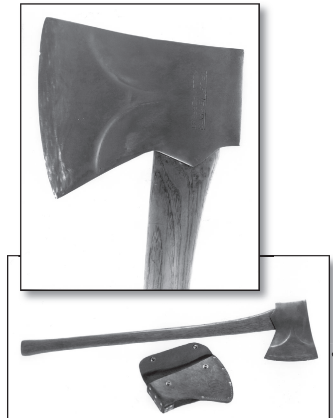
Figure 13—My favorite American felling ax, a True Temper Kelly Perfect with a Jersey head and 32-inch straight hickory handle. The scabbard is also shown.
