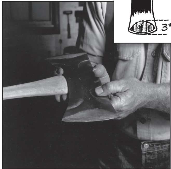
Figure 66—When sharpening, try for a fan-shaped effect on the cheek of the ax (drawing by Frederic H. Kock).
