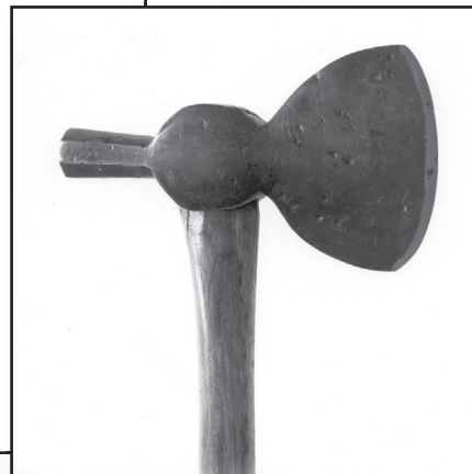
Figure 7—An 18th-century shingling hatchet is another specialized ax. Ax head is 5½ inches long by 4 inches wide.
