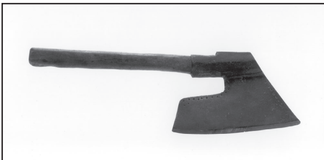
Figure 16—An 18th-century Germanic goose-wing hewing ax. The maker’s marks are hammered into the blade.
