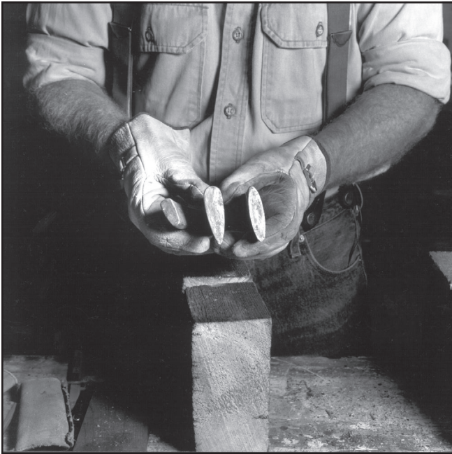
Figure 43—Use a wooden or steel drift or swedge to drive out the remainder of the handle. Notice the drift in the center is shaped for a single-bit ax, the one on the right is for a double-bit ax.
