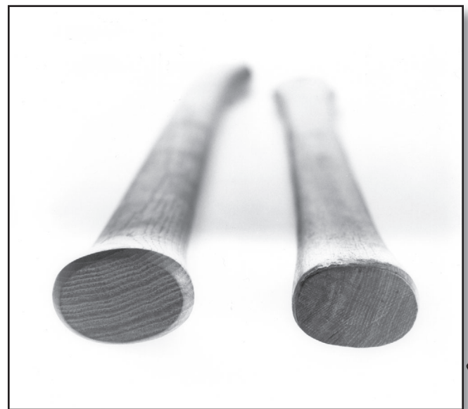
Figure 37—Grain orientation is important. The handle on the left has a good orientation. The one on the right does not, and is more likely to break under stress.
