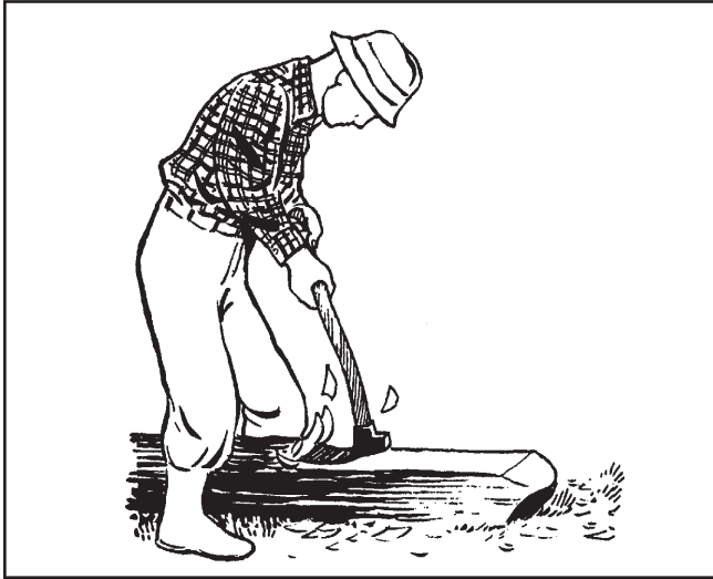
Figure 105—You may be able to straddle a small log when using an adz (drawing by Frederic H. Kock).
