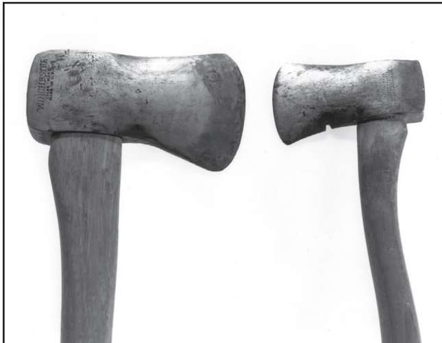
Figure 12—Winchester ax and hatchet, Michigan pattern, typical of the American felling ax.
