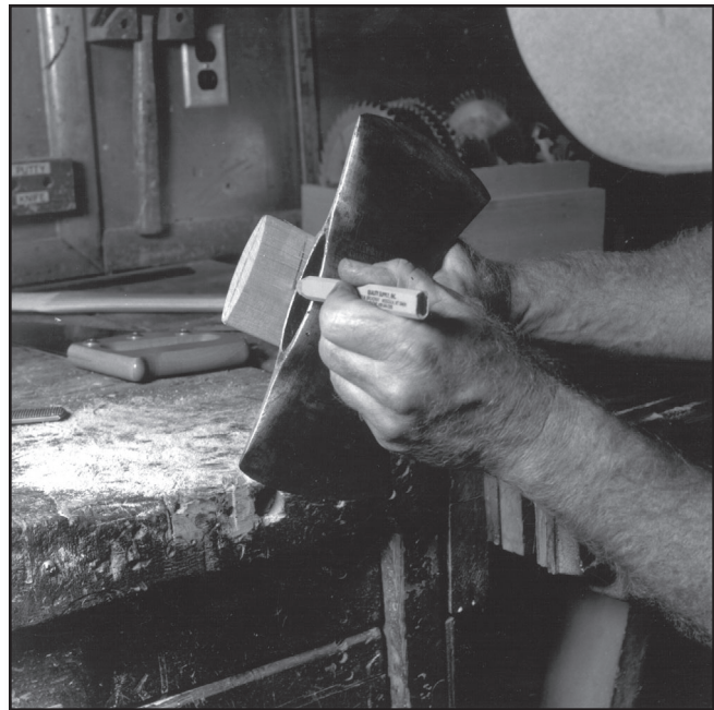
Figure 46—Take the new handle and place it next to the ax head. Bring the shoulder of the new handle all the way up to the bottom of the ax eye in its finished mounting location. This usually leaves quite a bit of excess wood on top. Draw a line to show where the excess wood should be cut off.
