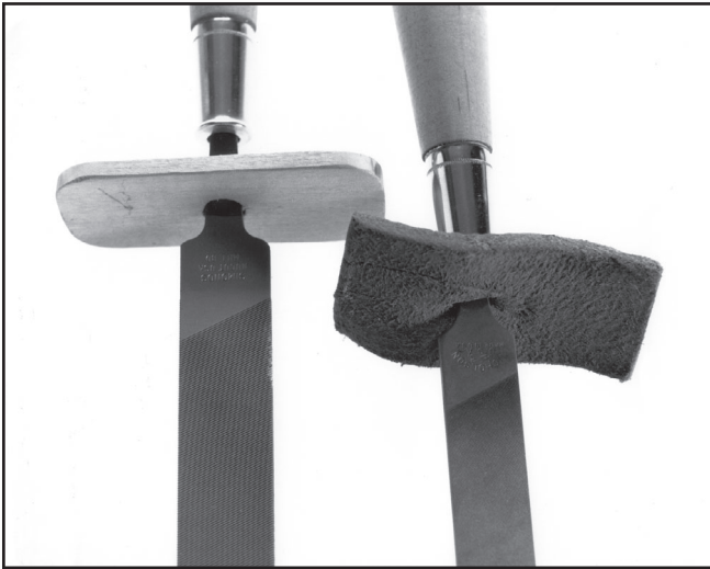
Figure 64—File guards help keep your fingers away from the sharpened ax blade.
