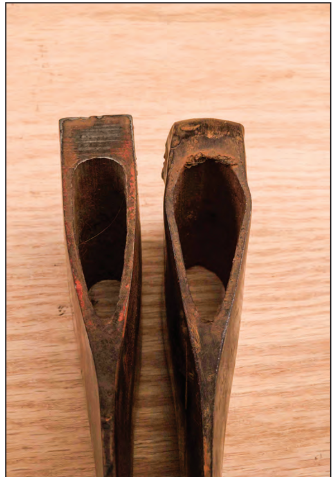
Figure 13–6—A properly shaped ax head eye (left) beside a misshapen ax head eye (right).
