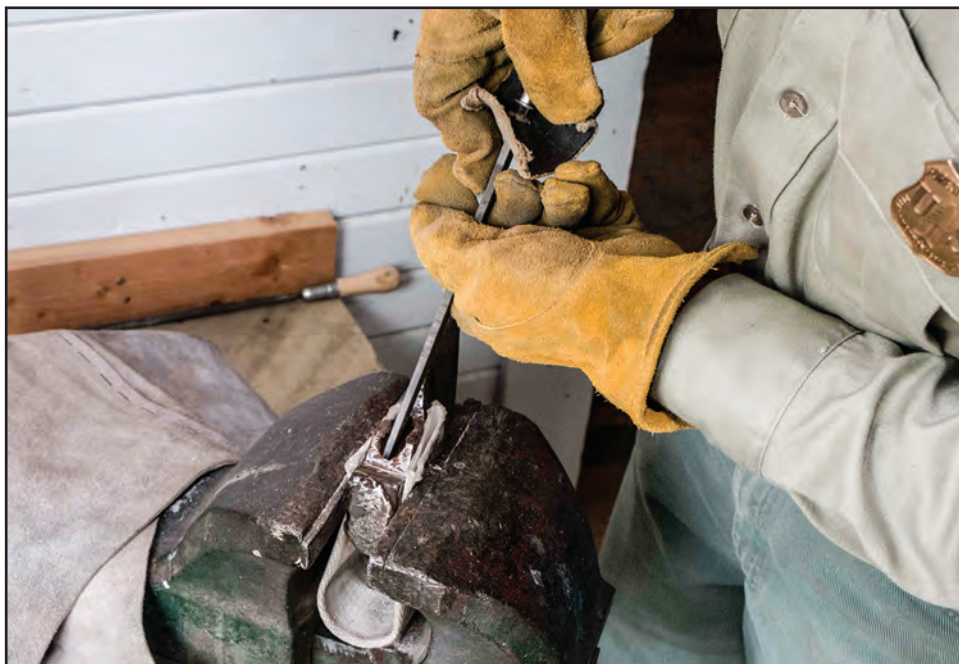
Figure 13–17—Filing off minor mushrooming on the inside of an ax head eye. Note that a flat file works best on the sides of the eye (right) and a round file works best on the rounded ends (below).
