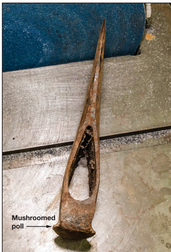
Figure 13-16—The photo above shows major mushrooming on a poll. The top photo on the following page shows someone grinding down the poll using a disc sander. The bottom photo on the following page shows the reshaped (reprofiled) poll.
