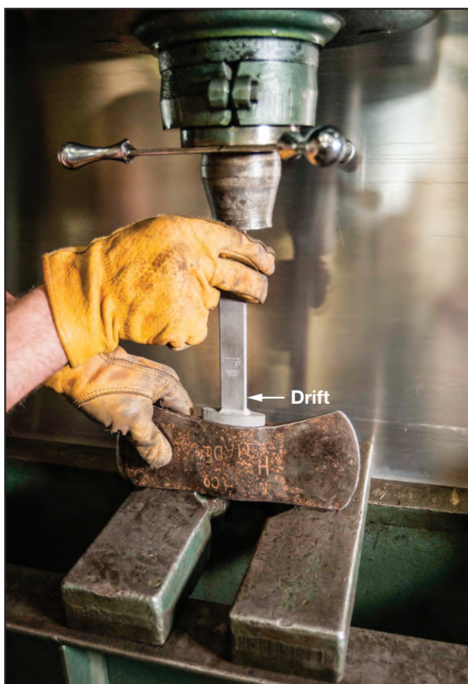
Figure 3-15—Using a drift pin to reshape an ax head eye.
