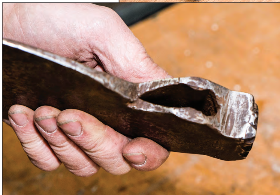
Figure 13-8—Distortion around the bottom of an L&J White broad hatchet head eye. This kind of damage usually occurs when someone tries to remove a handle using a hammer.
