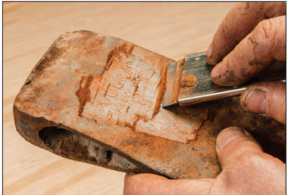
Figure 13–11 — Using a razor blade scraper to remove rust from an ax head.
