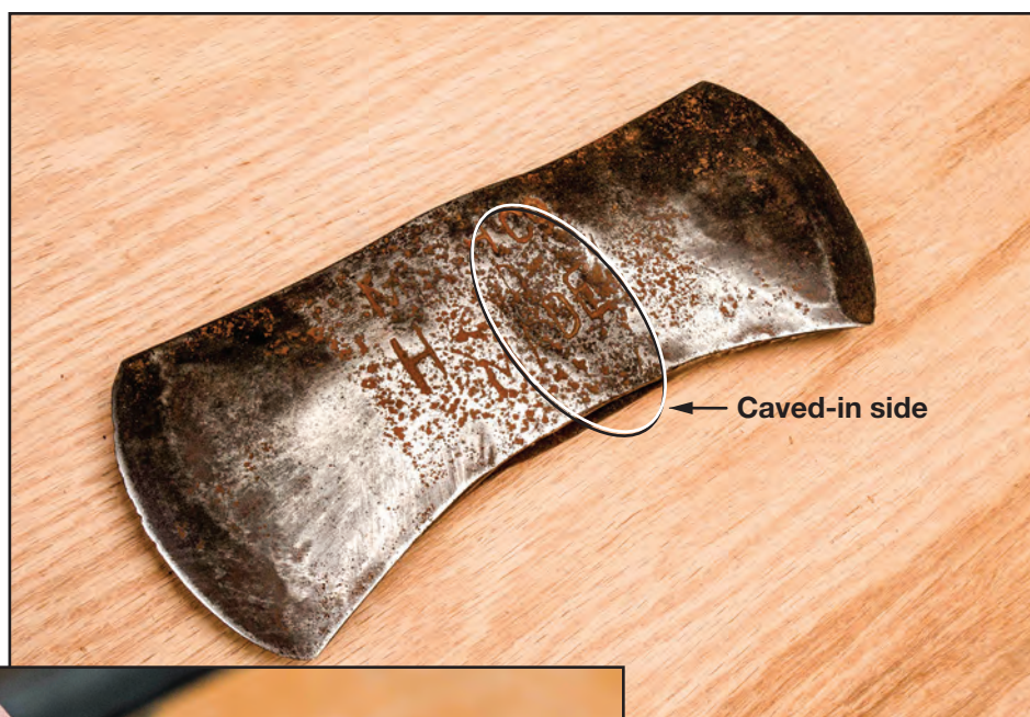
Figure 13-7—The eye of this Marshall Wells double-bit ax has caved-in sides.
