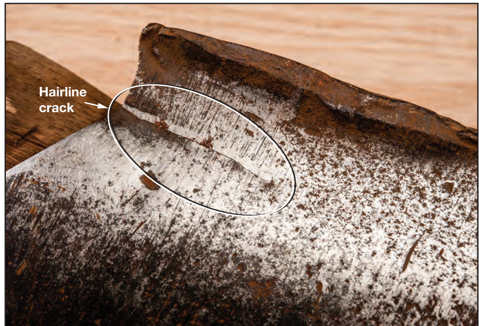
Figure 13–9—A hairline crack in an ax head.
