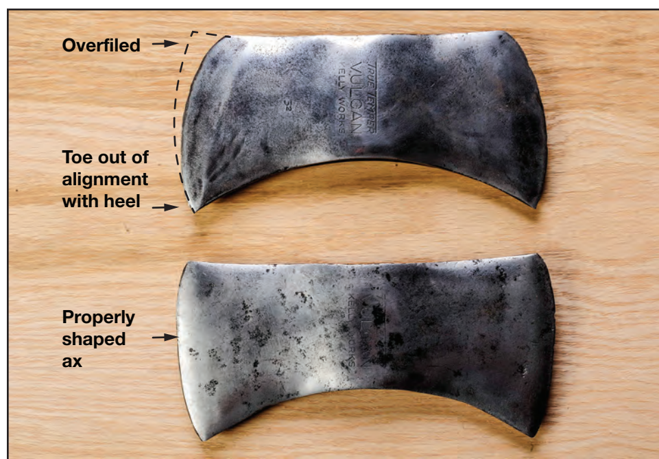
Figure 13–1—Two double-bit ax heads. The toe of the ax head on top has been filed out of alignment with the heel.
