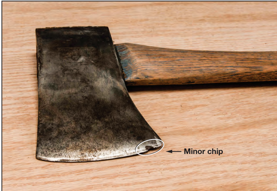
Figure 13-2—A minor chip in an ax head (left) and a major chip in an ax head (below).
