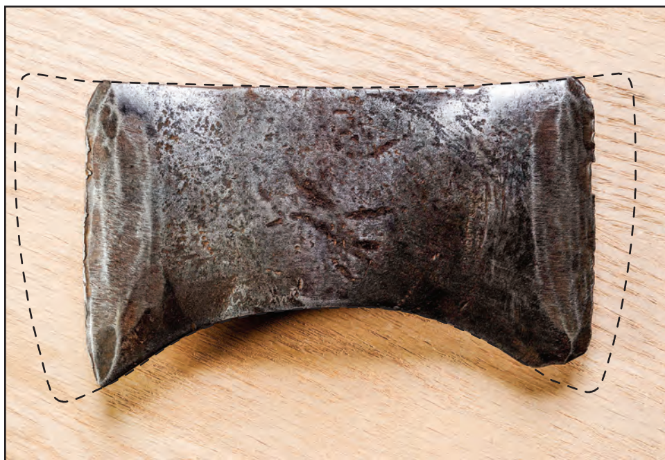
Figure 13–4—A Hubbard Lipincott double-bit ax head that has been filed past its temper line on both cutting edges. This head cannot be restored.
