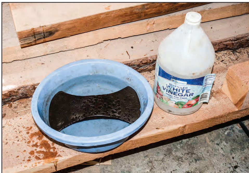
Figure 13-13—Soaking an ax head in white vinegar to remove the rust.
