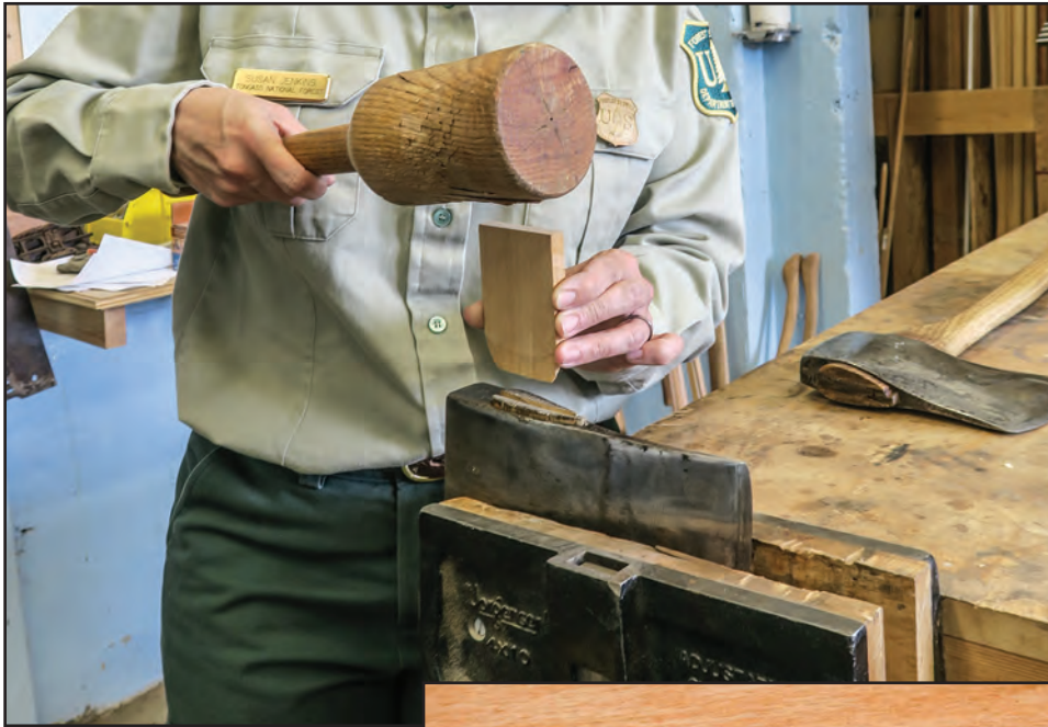
Figure 12-6—Using a new, thick wooden wedge and a mallet to tighten a loose ax head.
