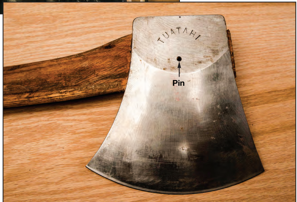
Figure 12-7—An ax head pinned to a handle.
