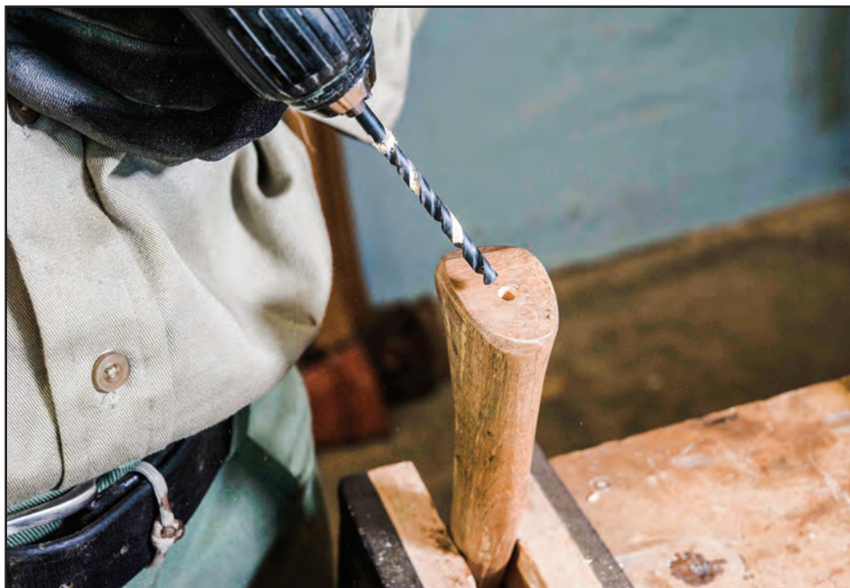
Figure 12-4—Drilling a small hole into the knob of an ax handle and filling the hole with linseed oil enables the handle to absorb the oil over time.
