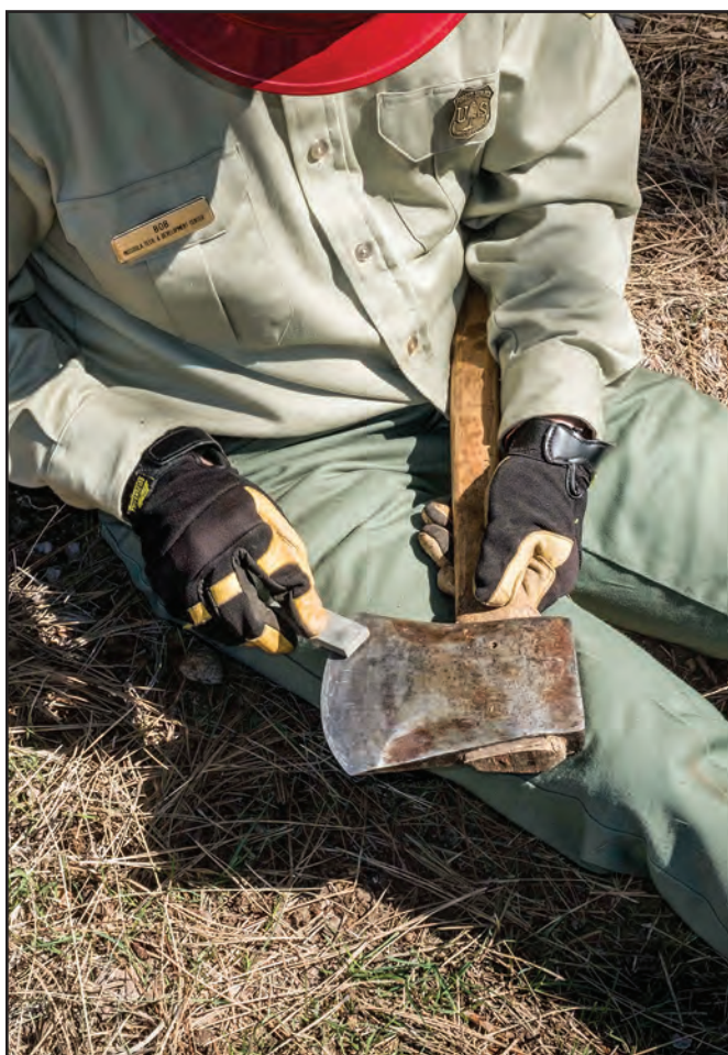
Figure 12-1—Running a fine whetstone along a cutting edge.
