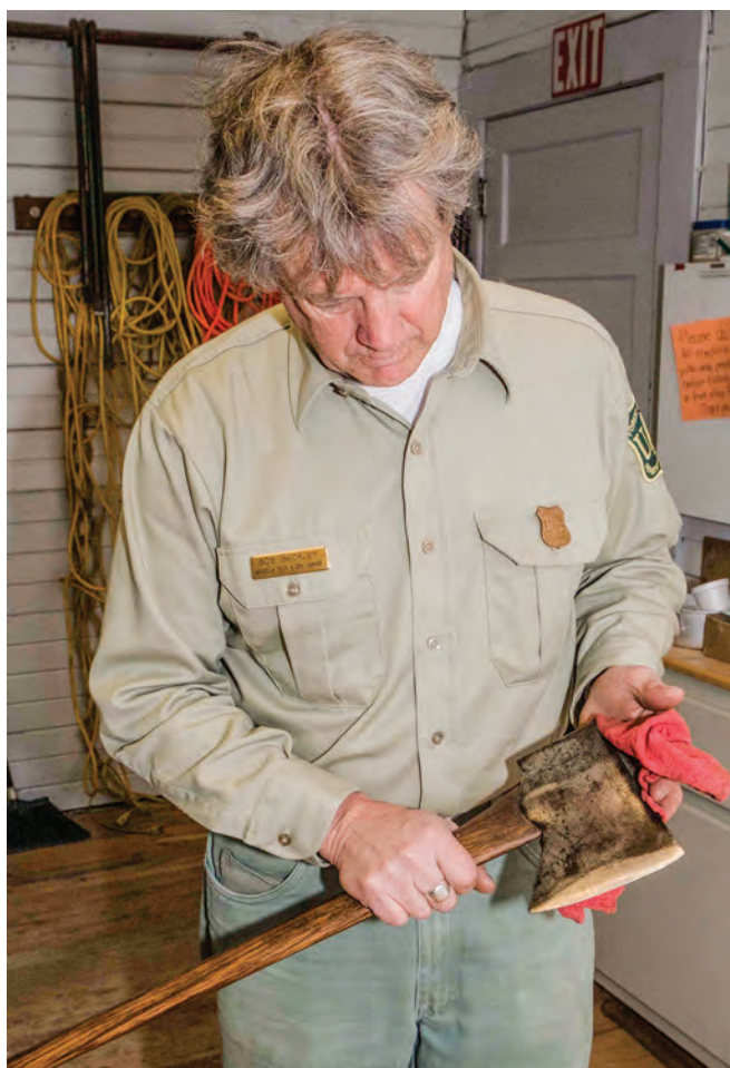
Figure 12-2—Cleaning an ax head with a rag.
