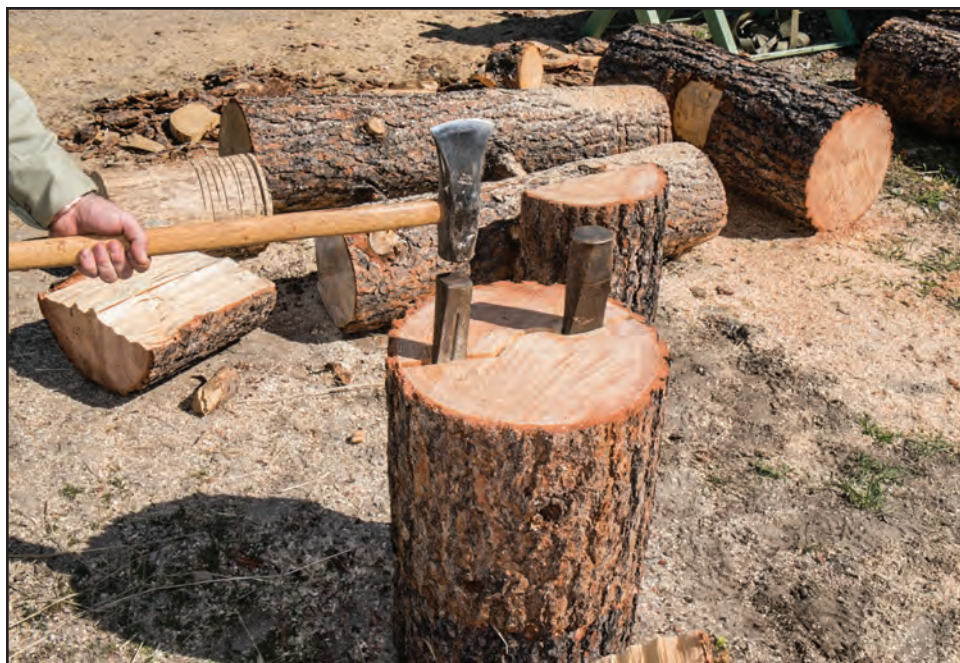
Figure 11-78—Striking a wedge with a maul after driving a wedge into the opposite side of the round.
