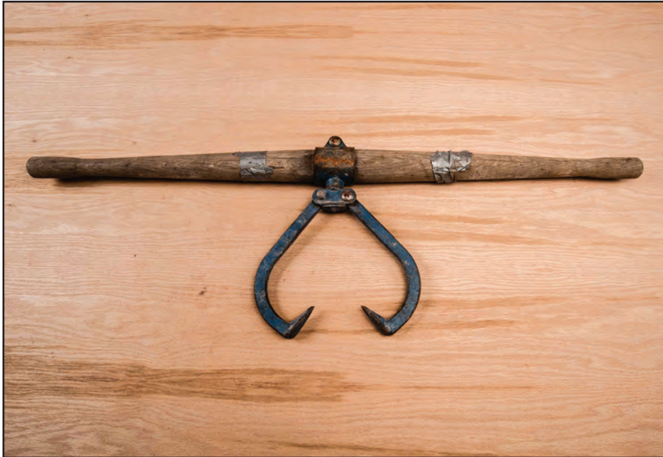
Figure 11–62—A log carrier designed for two people.
