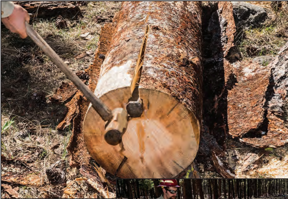
Figure 11-79—Using a sledge hammer and wedge to split a rail from a log.
