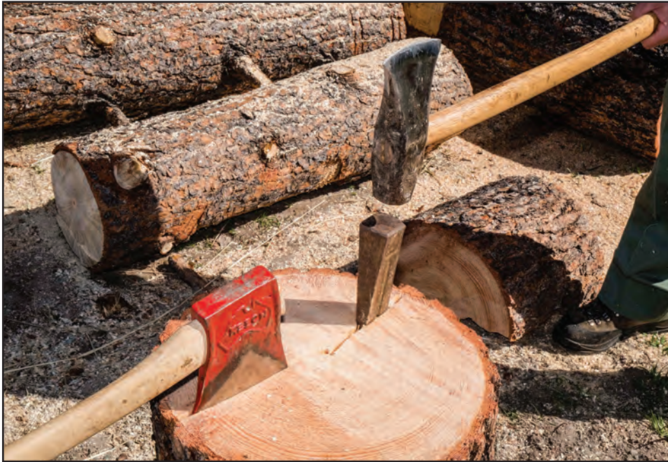
Figure 11-75—Using a wedge and maul to split a round and free a bound ax. An ax is more likely to bind when striking the center of a round. Striking the edge of a round not only decreases the likelihood that the ax will bind, but also splits the round more easily.
