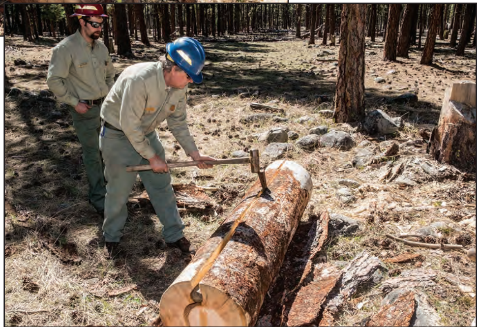
Figure 11-80—As the split in figure 11-79 develops, drive another wedge into the split.
