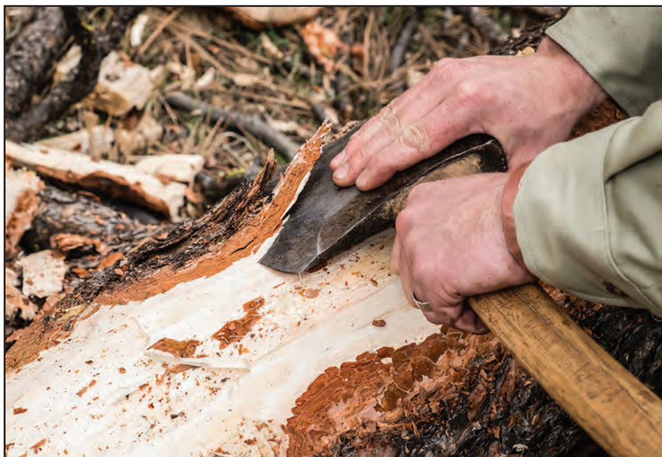
Figure 11–85—Removing bark with an ax blade. Note the shallow angle of the blade in relation to the log.
