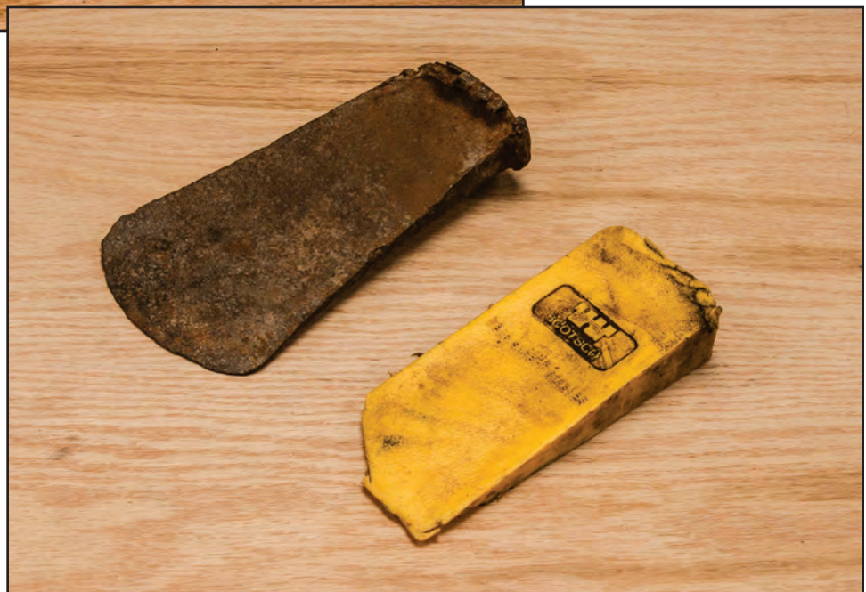
Figure 11-53—Mushroomed and damaged felling wedges.
