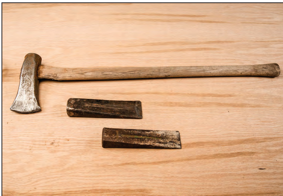
Figure 11–68—A maul and splitting wedges.
