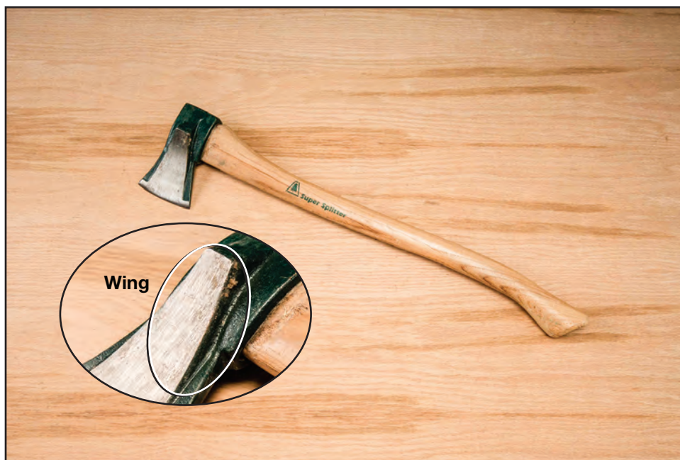
Figure 11-71—A modern splitting ax with wings that help spread and split the log. The inset shows a closeup of one wing.
