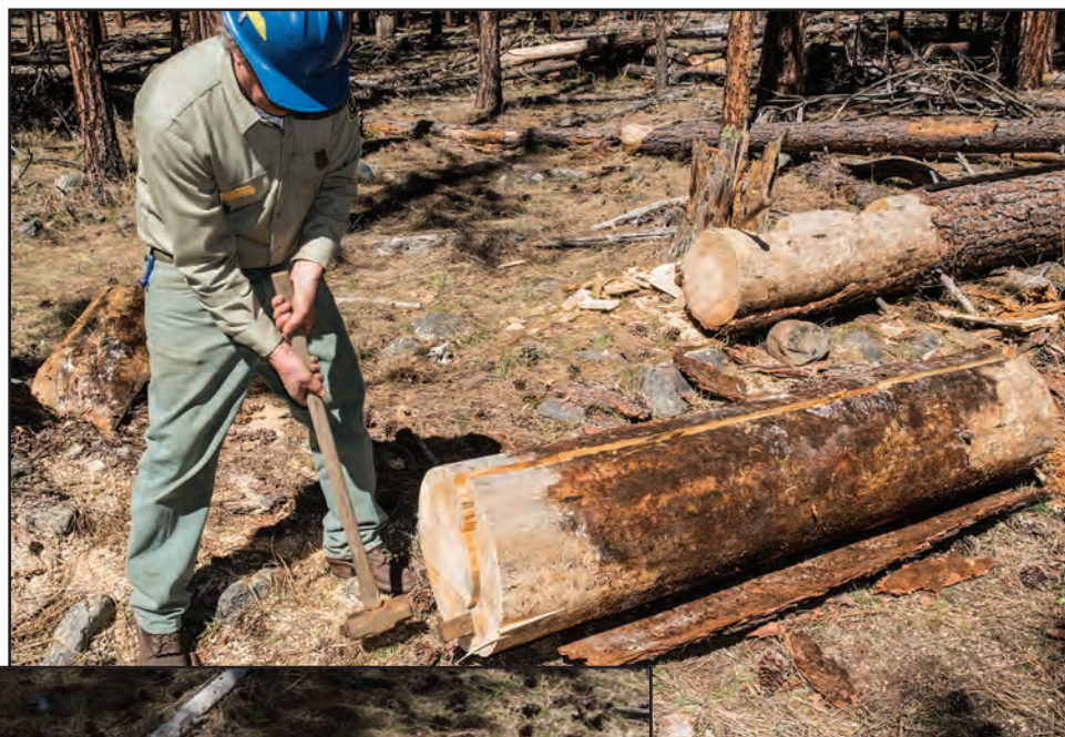
Figure 11–81 — Continue to drive wedges down the length of the log until the log splits.
