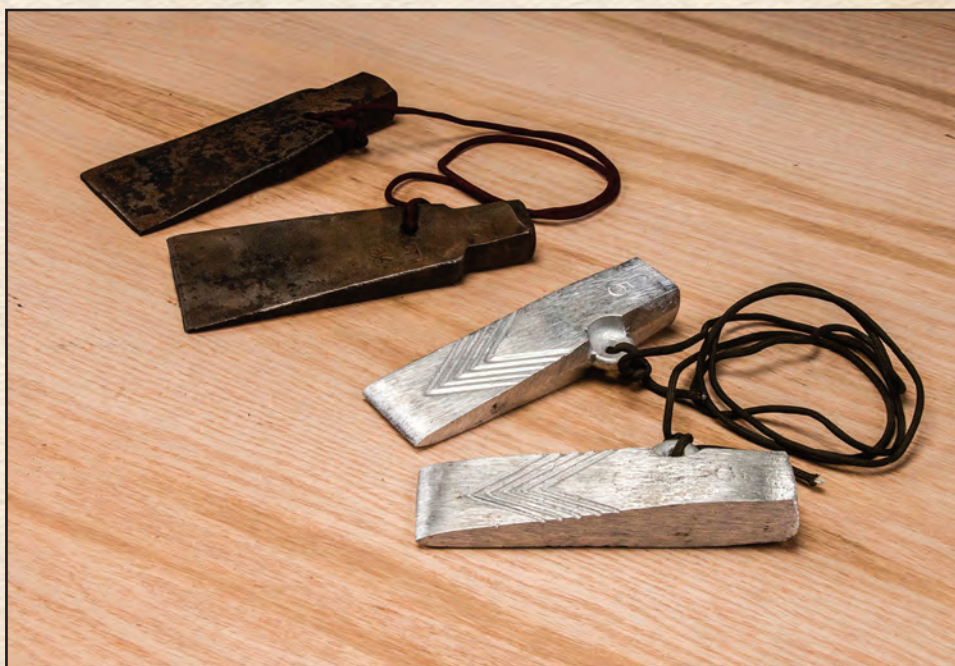
Figure 11-56—Newly manufactured aluminum holding wedges (foreground) tend to be thicker than vintage holding wedges (background).
