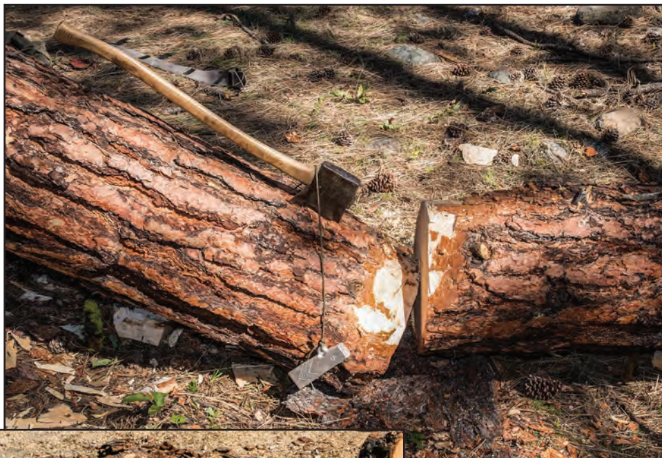
Figure 11–58—With the lanyard connecting the wedges over the back of the lodged ax head, the wedges remain fixed on the log after the cut end of the log drops away.
