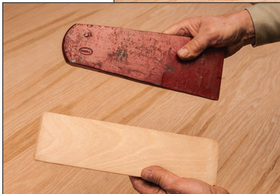
Figure 11–51—A steel wedge (top) and a wooden wedge (bottom).
