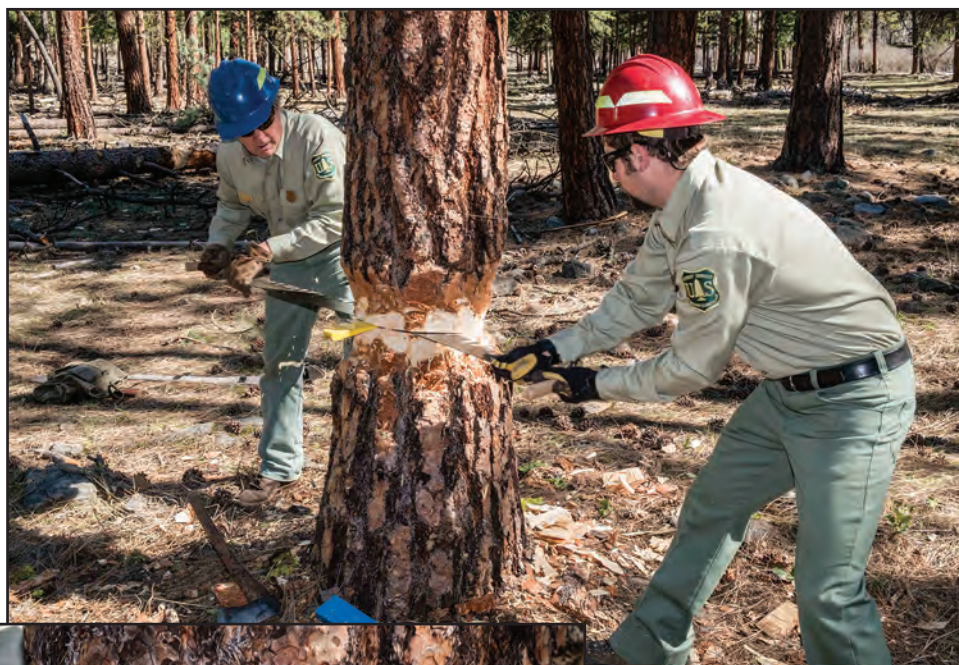
Figure 11–44—Performing a back cut on a tree using a crosscut saw.
