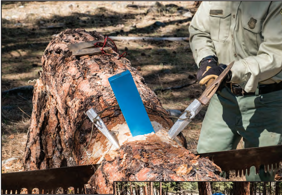
Figure 11–57—Driving wedges into a log (left). Note the lanyard placed over the back of the ax head (below).
