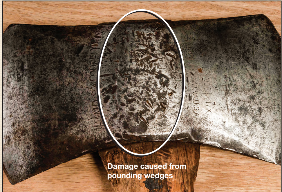
Figure 11–69—Driving wedges with a double-bit ax can damage the sides of the ax head.
