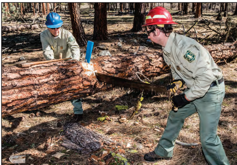
Figure 11–55—Using a wedge to hold a kerf open on a log.
