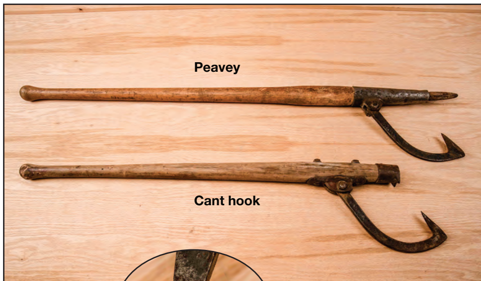
Figure 11–66—A peavey and cant hook. Note the spike on the peavey and the dogs (teeth) and the hook on the cant hook.
