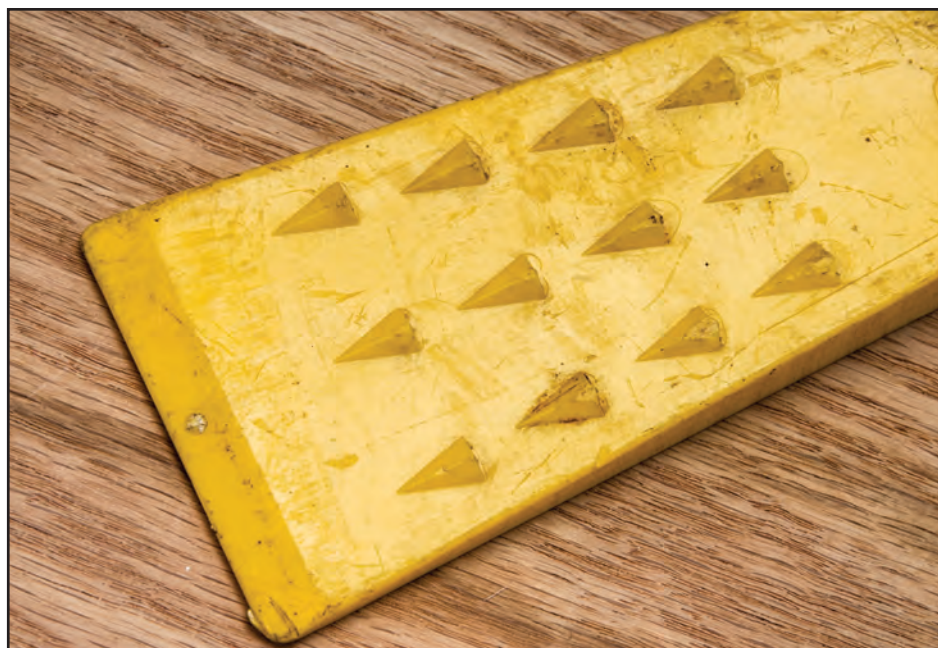
Figure 11-54—A wedge with a ridged surface.
