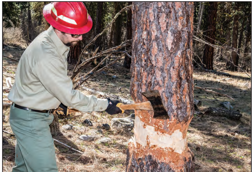
Figure 11–49—Clearing bark from an area on a tree before using a crosscut saw.
