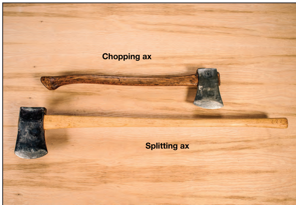
Figure 11-70—A 4½-pound Arvika 5-Star ax head on a 27-inch handle (top) and a 5¾-pound American Axe and Tool Company ax head on a 44-inch handle (bottom).
