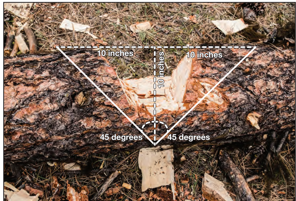
Figure 11–21—This notch is too narrow to continue removing big chips; it must be wider to enable the ax to cut through to the bottom of the log.
