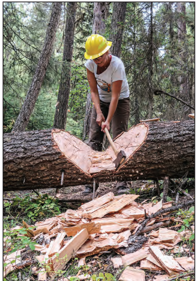
Figure 11–14—An ax blade penetrating deep enough into wood to cause wedging action and to displace wood chips. Note the size of the wood chips; they indicate a well shaped ax and proper chopping technique.
