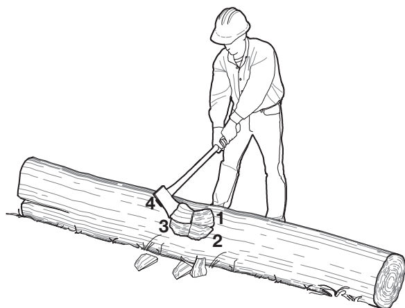
Figure 11–19—Chopping in either sequence shown will clear chips from the top portion of the log, making the bottom portion visible and reducing the chance of striking the ground with the ax.
