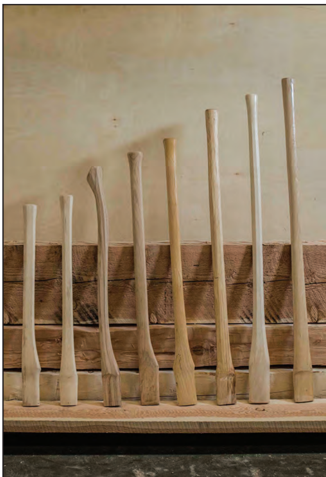
Figure 11–26—Various sizes of ax handle, ranging from 26 inches to 44 inches.
