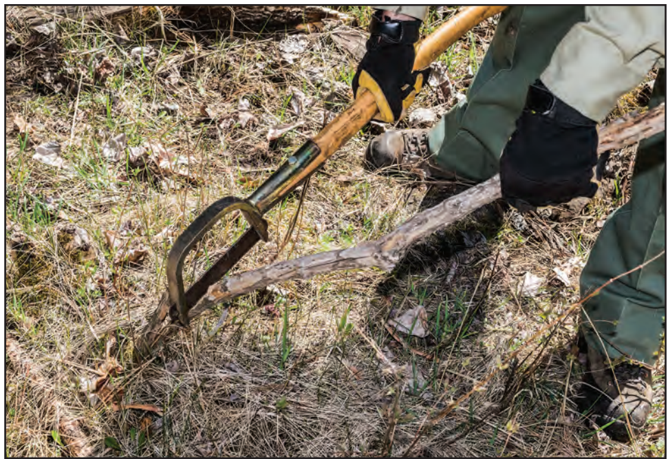
Figure 11-29—Using a Swede ax to cut a dead sapling.
