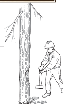
Figure 11–15—An ax head chopping at a 45-degree angle, severing wood fibers and releasing wood chips. A closeup view (inset) of the driving force of the ax head, the wedging force to either side of the ax head, and a high-stress point at the cutting edge of the ax head where the wood chips release.
