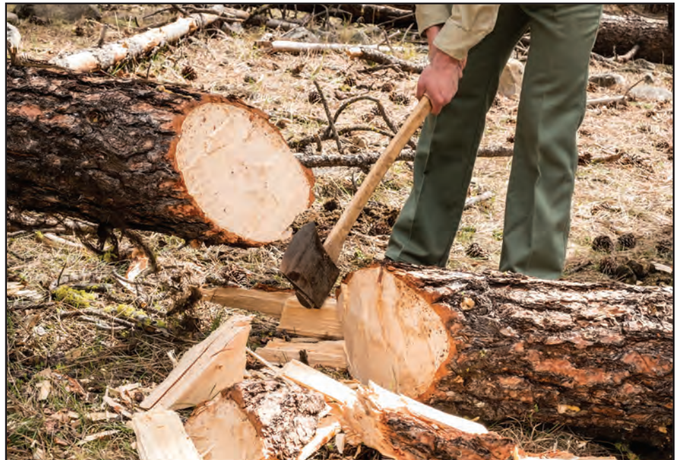
Figure 11–32—Using the poll of an ax to break through a log.
