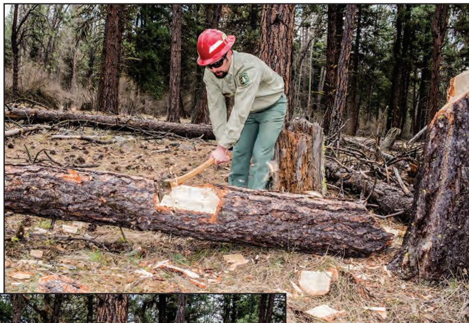
Figure 11-25—Squaring the shoulders and hips in line with the ax stroke. Note that the axman in these pictures has turned his body to be in line with his chop.
