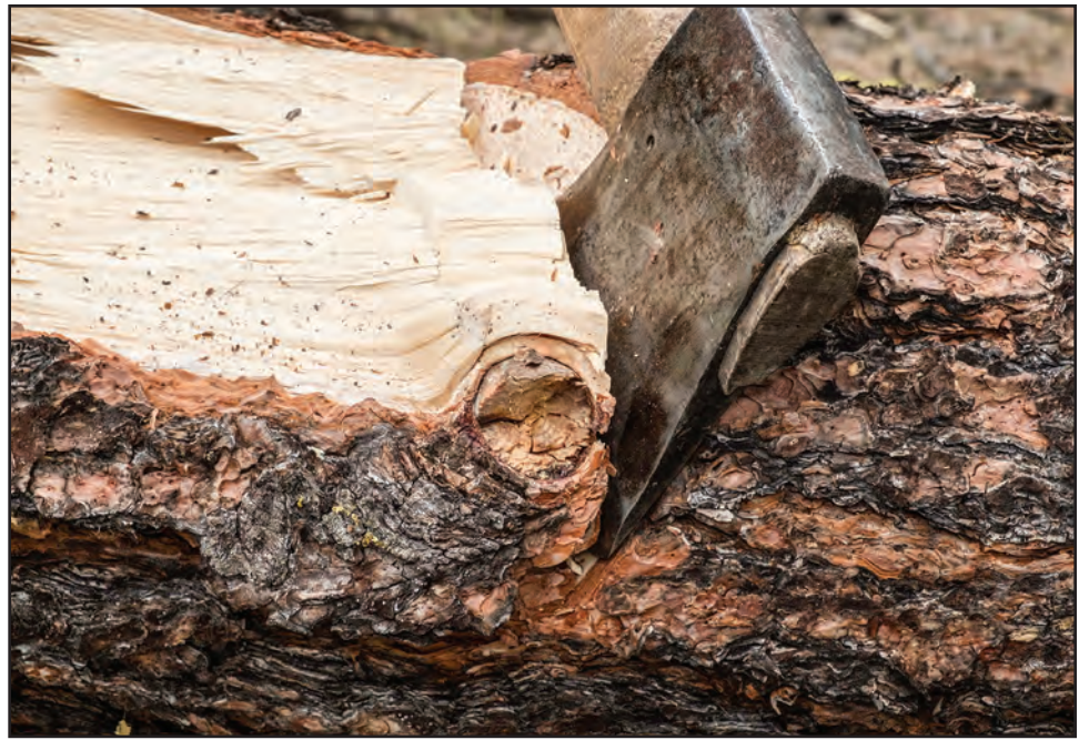
Figure 11–24—Cutting around a knot in a log.
