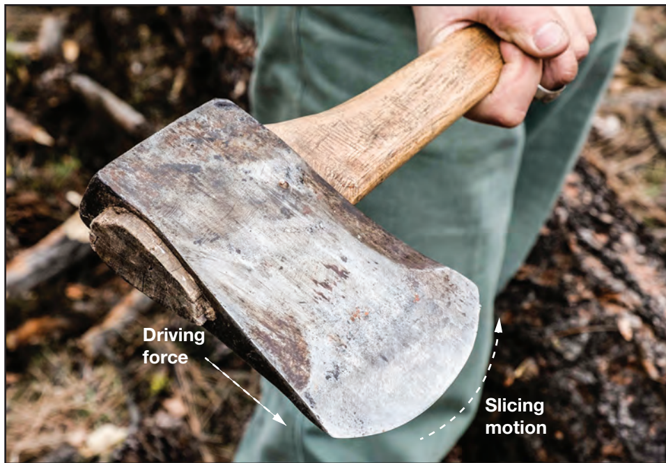
Figure 11–13—The arrows in this picture indicate how the cutting edge of an ax head slices through and severs wood fibers and how the driving force helps to pop out the wood chip.
