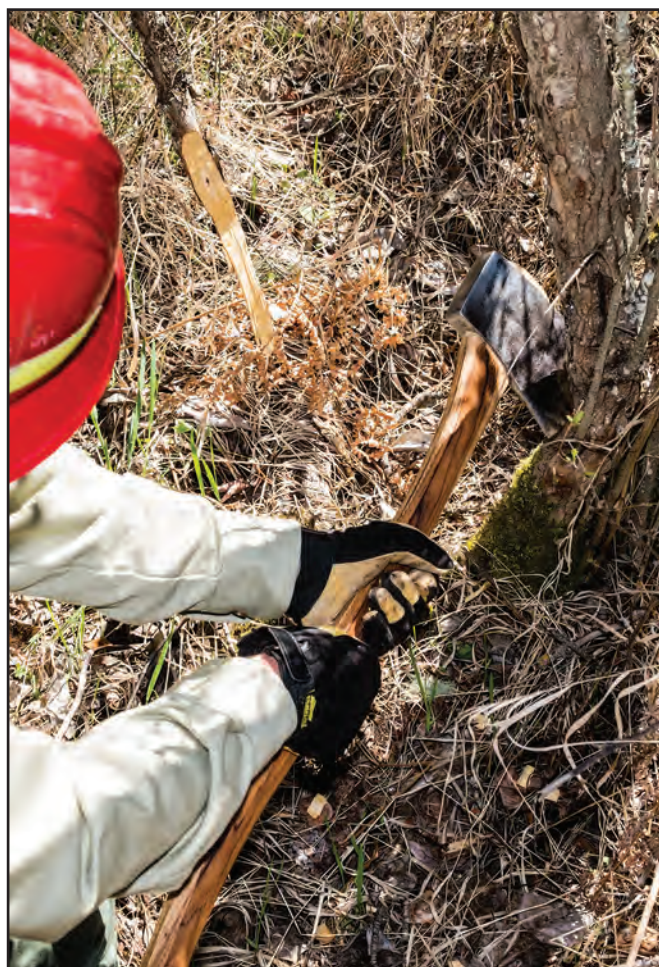
Figure 11–27—A choked grip makes it easier to cut brush, though there may be other tools that are more appropriate for the job, such as lopping shears or a small pruning saw.
