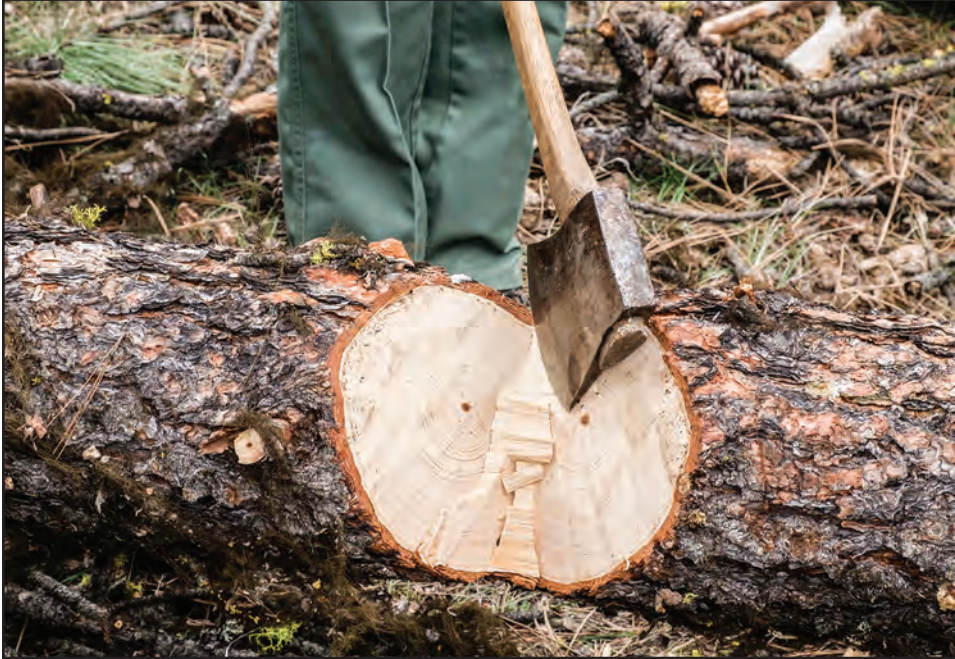
Figure 11–20—When chopping from only one side of a log, make sure to cut the notch twice the diameter of the log.
