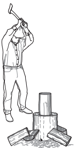
Figure 11–14—An ax blade penetrating deep enough into wood to cause wedging action and to displace wood chips. Note the size of the wood chips; they indicate a well shaped ax and proper chopping technique.
