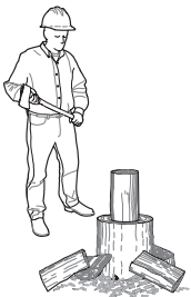
Figure 11-17—Holding an ax with one hand on the throat and the other hand on the shoulder.
