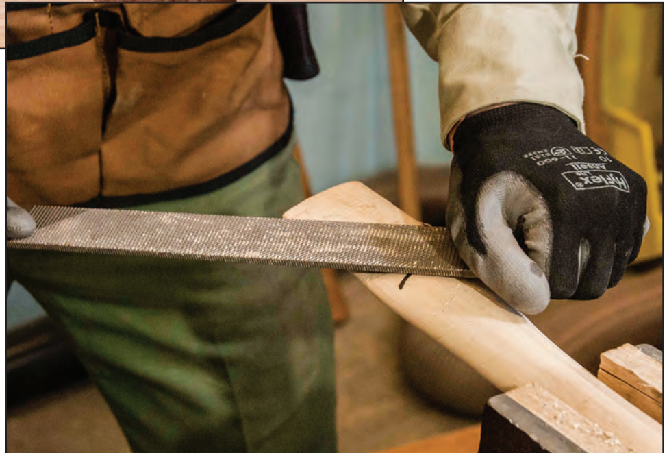
Figure 10-8—Using a rasp to remove wood from an ax handle.
