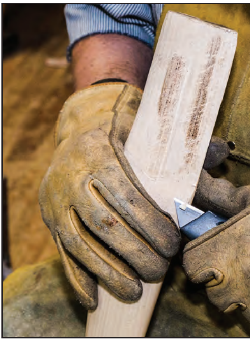
Figure 10-12—Removing wood from the leading edge of the handle where it sits inside the eye of the ax head.
