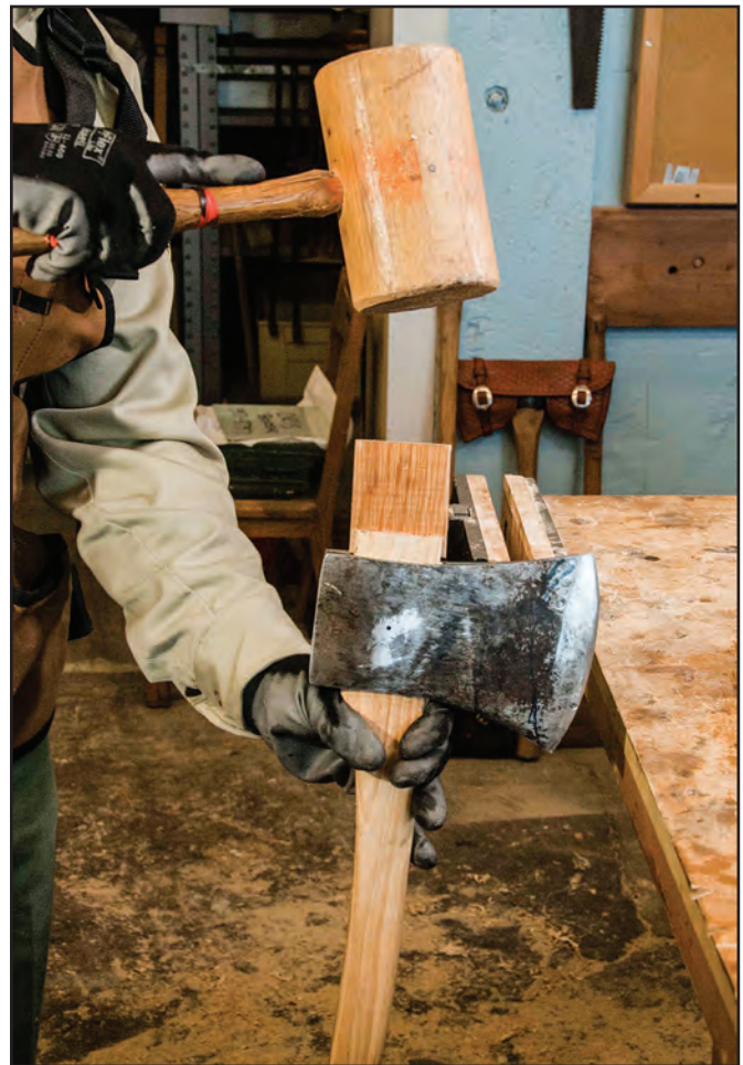
Figure 10–16—Using a wooden mallet to drive the wedge into the ax handle kerf.
