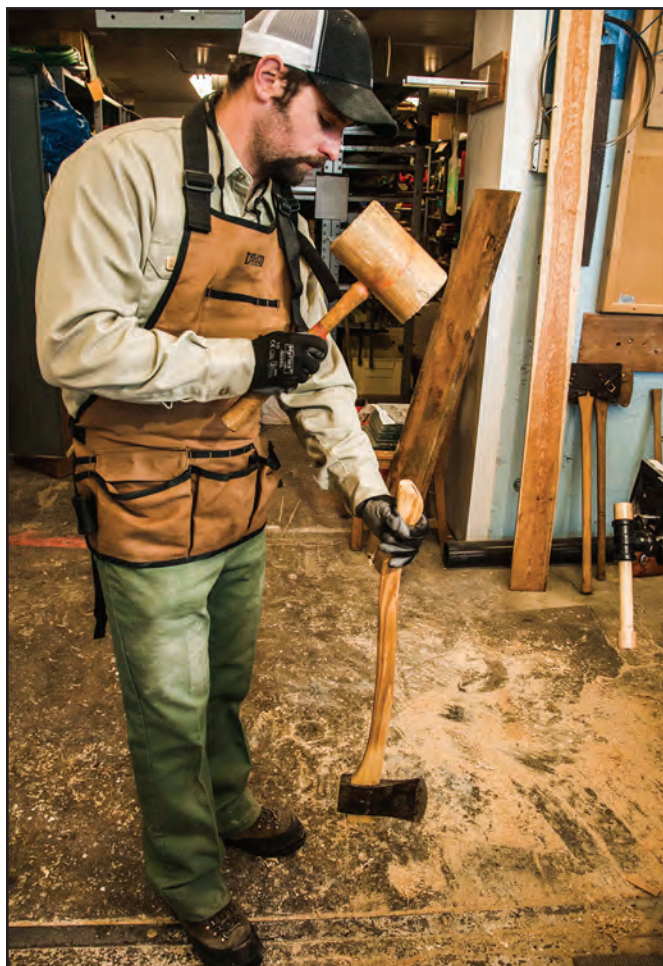
Figure 10–9—Strike the heel of the ax handle to draw the ax head onto the handle. Note that the fawn's foot on this handle has a flat bottom.
