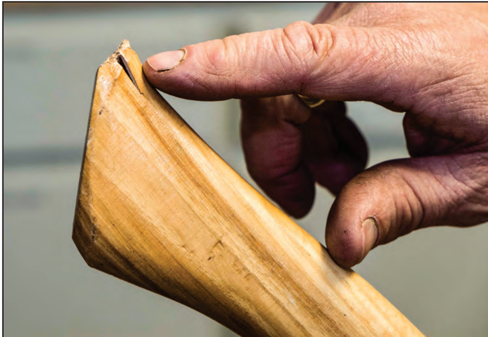
Figure 10–10—Repairing a curved, single-bit handle with a damaged heel (left) by removing about ½ inch of the handle (below) and smoothing the heel using sandpaper (facing page, top).
