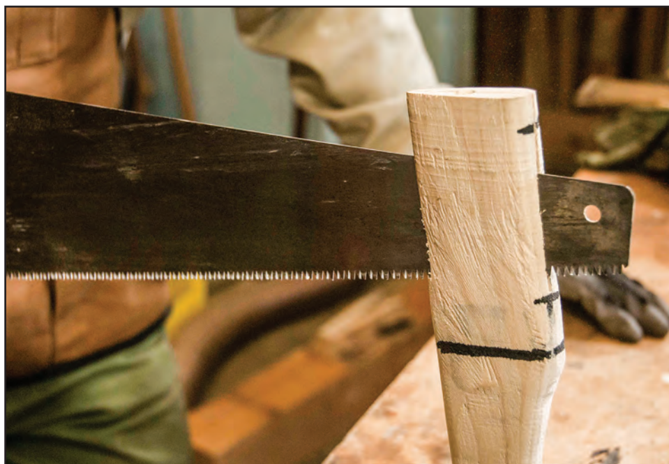
Figure 10-15—Using a handsaw to make the ax handle kerf deeper.
