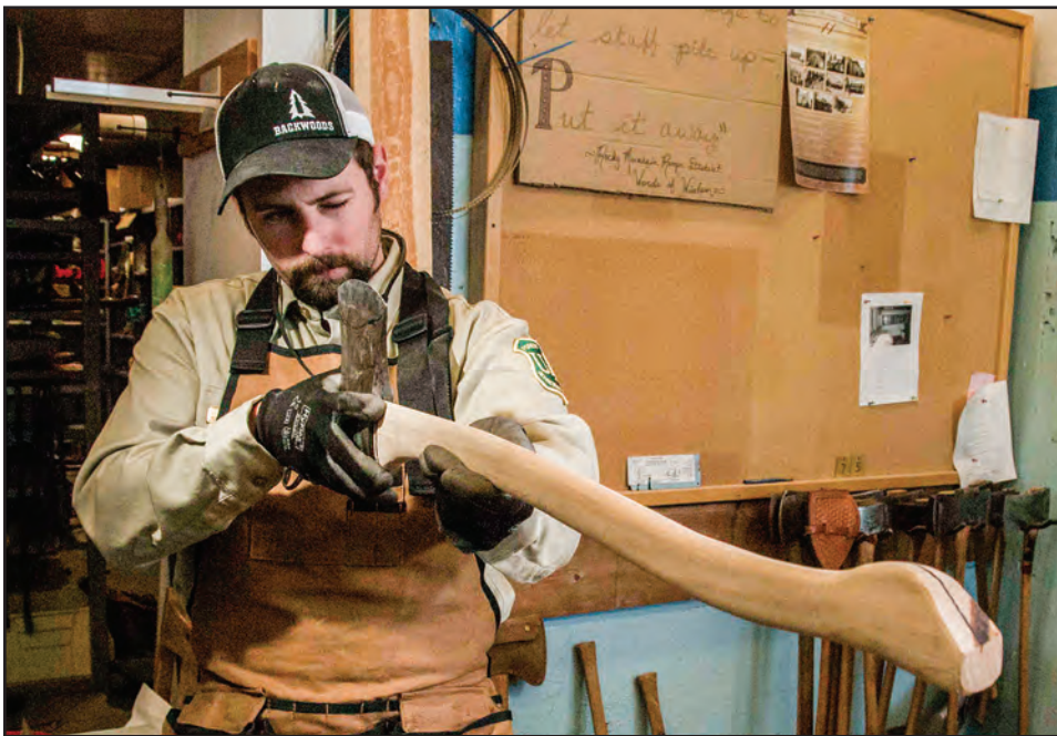
Figure 10-3—Sighting down the midpoint of the heel of the cutting edge to ensure that it aligns with the center of the knob on the handle.
