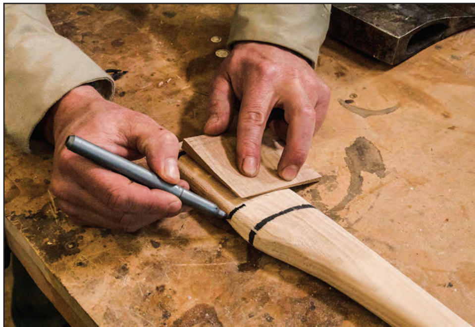
Figure 10-14—Marking the depth of the wedge to indicate how far it will reach into the kerf.
