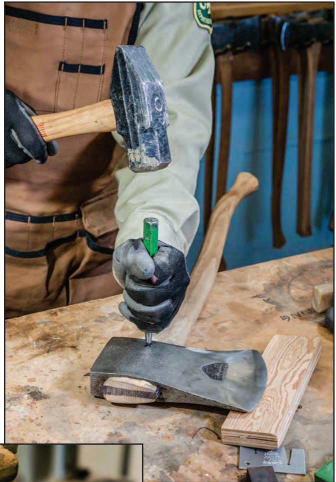
Figure 10–2—Using a center punch to mark an ax head to insert a pin (right), drilling a small hole through the ax head and handle (below and facing page, top), and driving a roll pin through the hole (facing page, bottom).
