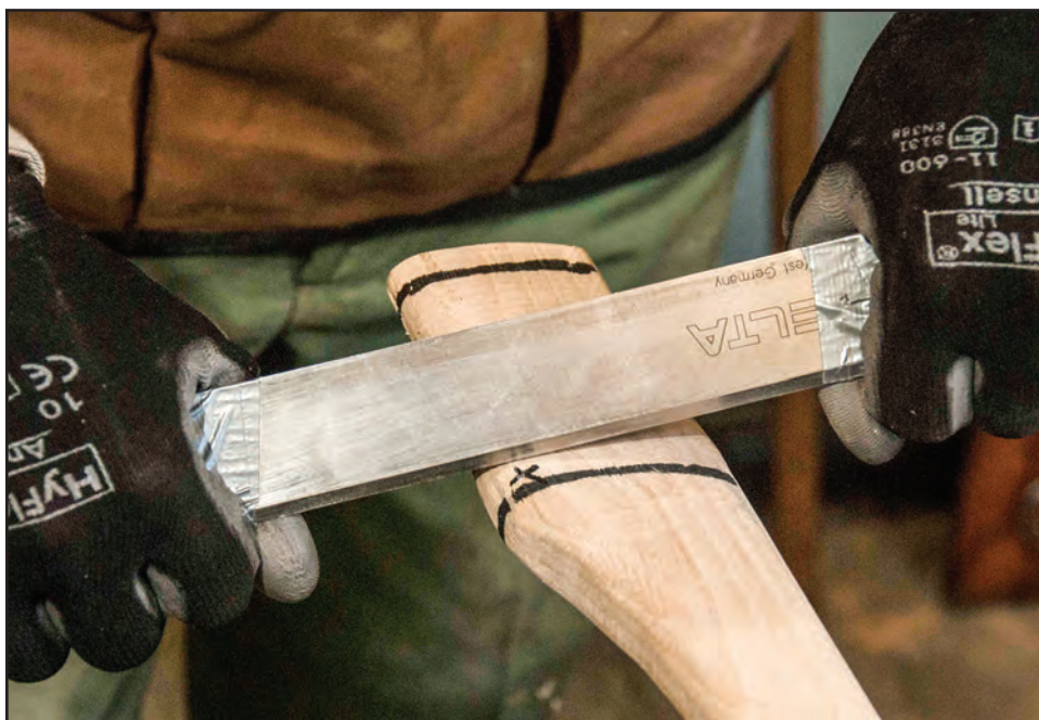
Figure 10-11 — Ensuring the lateral alignment of the ax head with the ax handle by removing wood from the handle where it sits inside the ax head eye.
