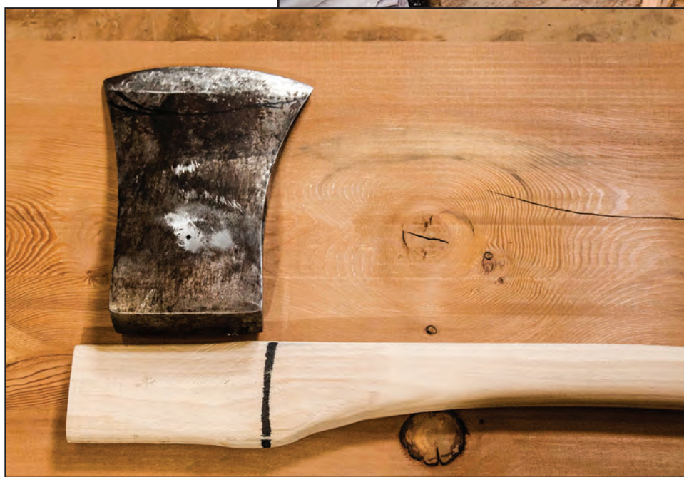
Figure 10-6—An ax head resting beside the shoulder of a handle.
