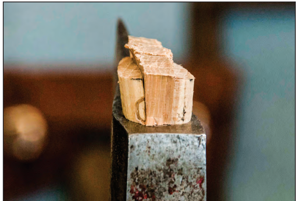
Figure 10–17—The wedge expands the top portion of the ax handle to grip the sides of the ax head eye.
