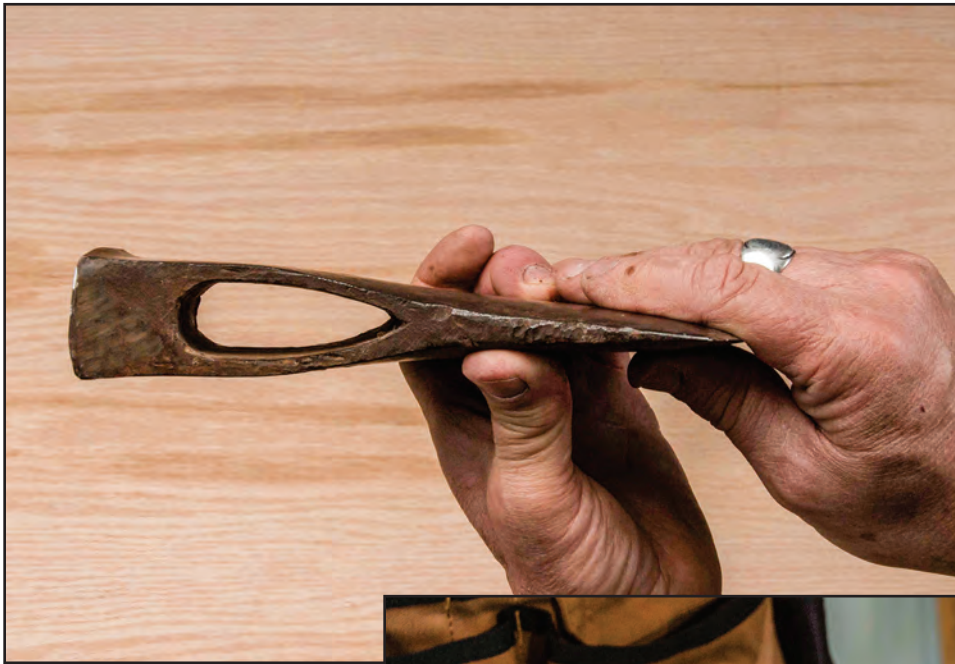
Figure 10-7—Looking through the top eye of an ax head. Note that the top of the eye is slightly larger than the bottom to allow for the placement of the wedge.
