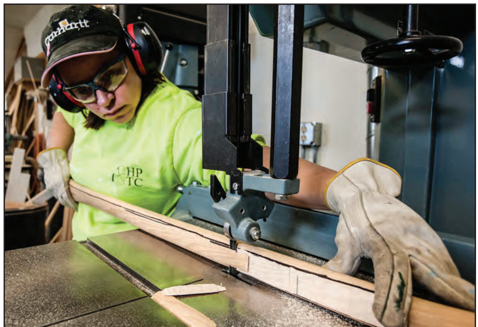
Figure 9-7—Using a band saw to thin down a thick handle.
