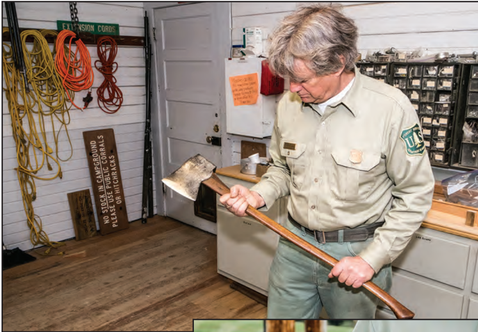
Figure 9–10—A properly shaped, thinned down handle. Note how the fingers overlap the handle.
