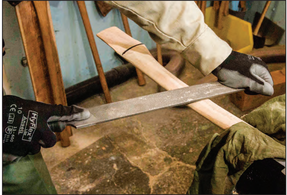
Figure 9–6—Using a rasp (left), a planer blade (below), and a spoke shave (following page, top) to shave wood from a handle secured in a vise on a workbench.
