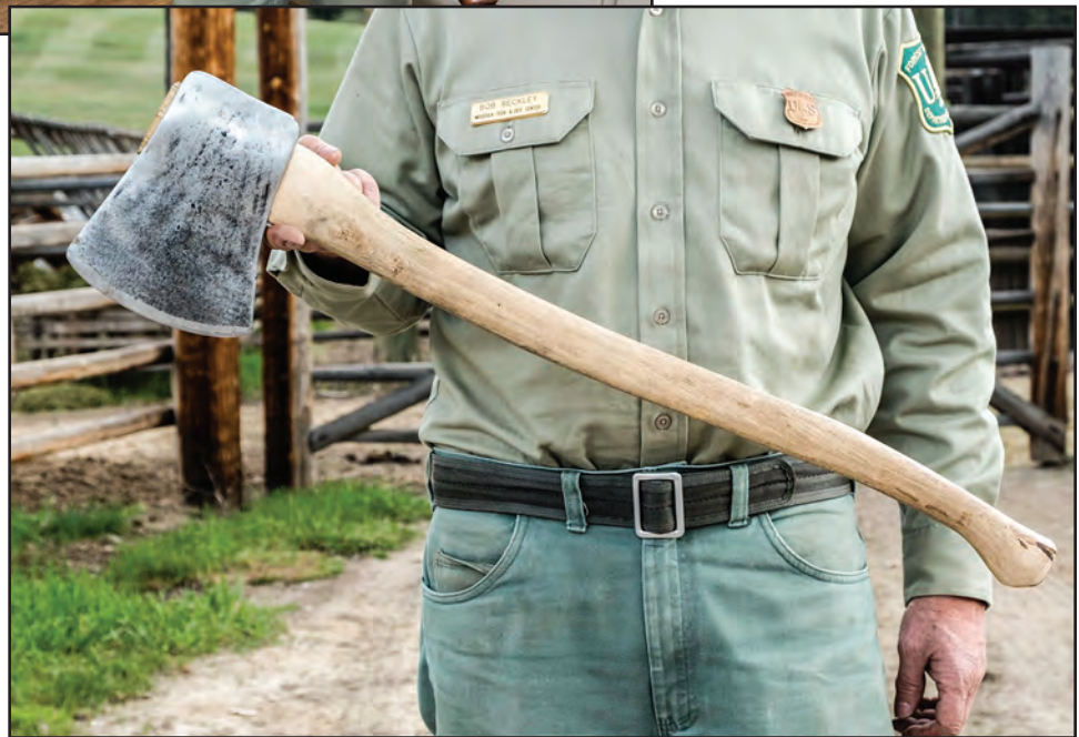
Figure 9–11—A properly balanced single-bit ax resting on one finger, indicating that the balancing point is close to the ax head.
