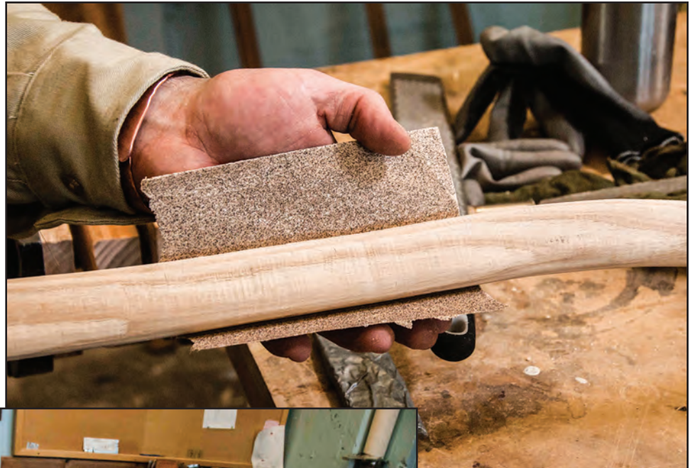
Figure 9-12—Sanding down an ax handle to make it smooth.
