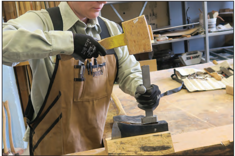
Figure 9-4—Using a mallet and drift pin to remove the remaining portion of a handle from an ax head eye.
