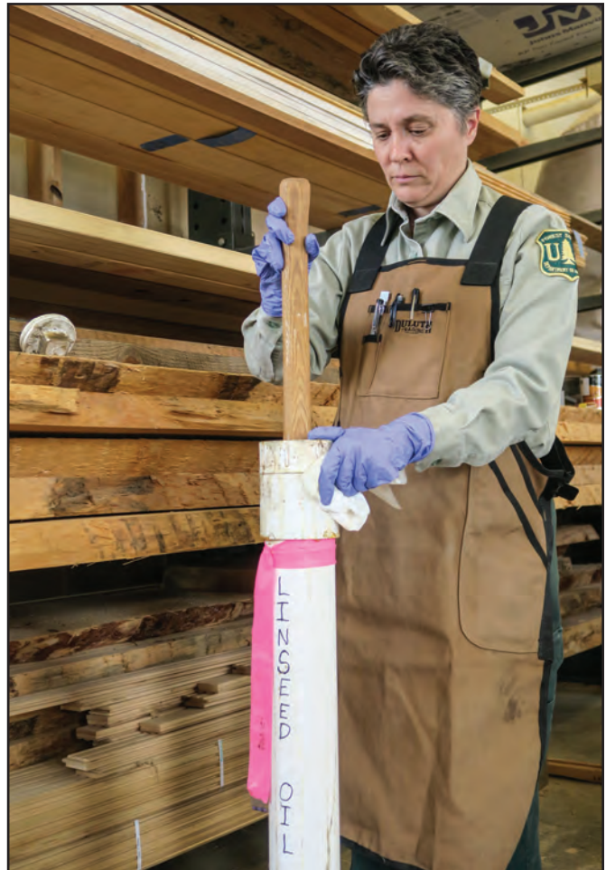
Figure 9–14—Removing an ax handle from polyvinyl chloride (PVC) pipe filled with linseed oil.
