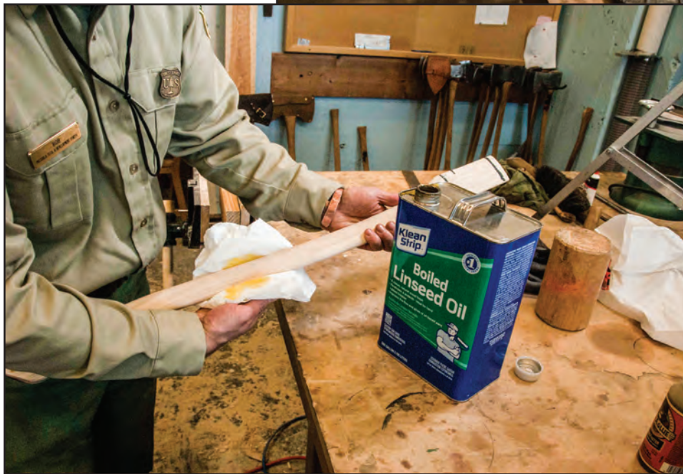
Figure 9-13—Rubbing boiled linseed oil into a handle to achieve a smooth finish.
