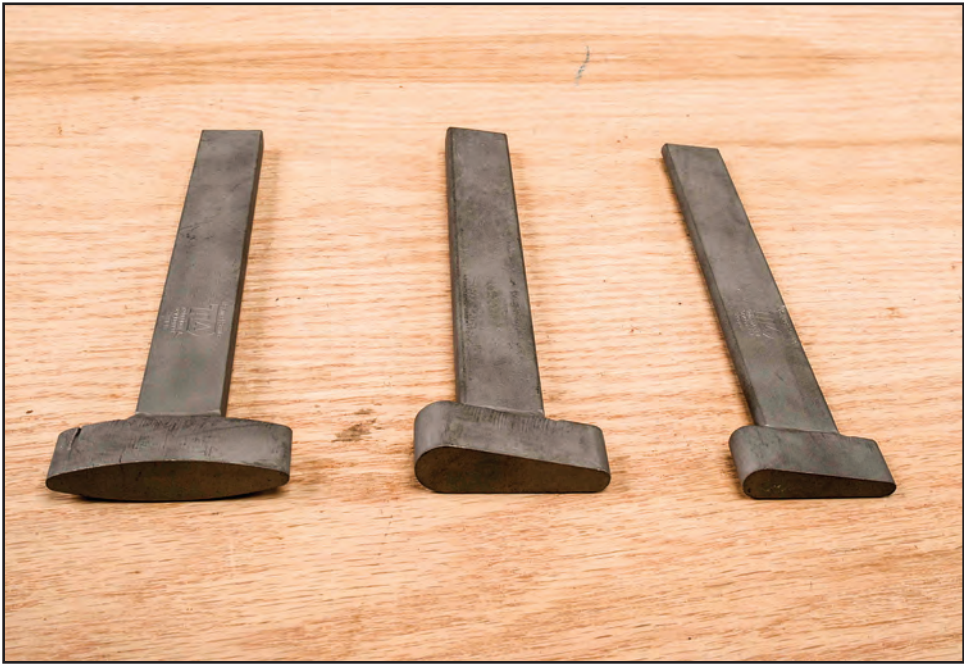
Figure 9-3—Three drift pins used for removing a handle from the eye of an ax head.
