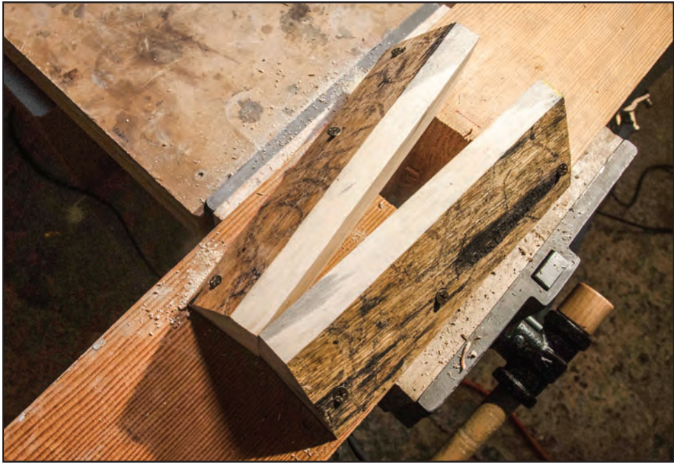
Figure 9-2—A simple bench-top jig secured by a vise.
