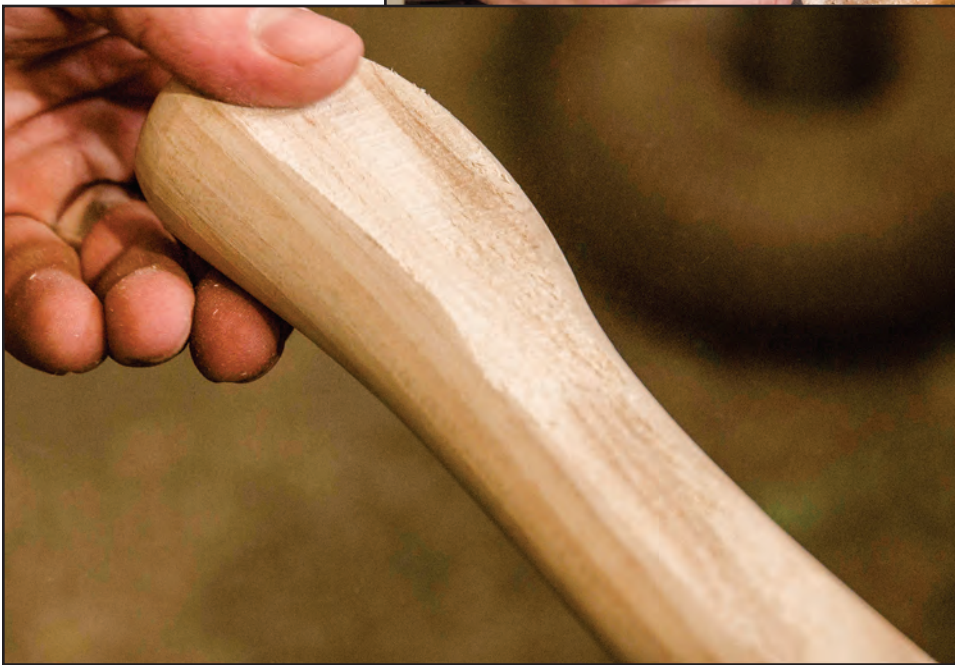
Figure 9–9—The throat and knob of an ax handle.
