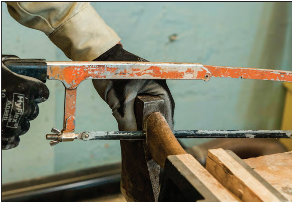
Figure 9–1—Sawing off a broken handle below the ax head.
