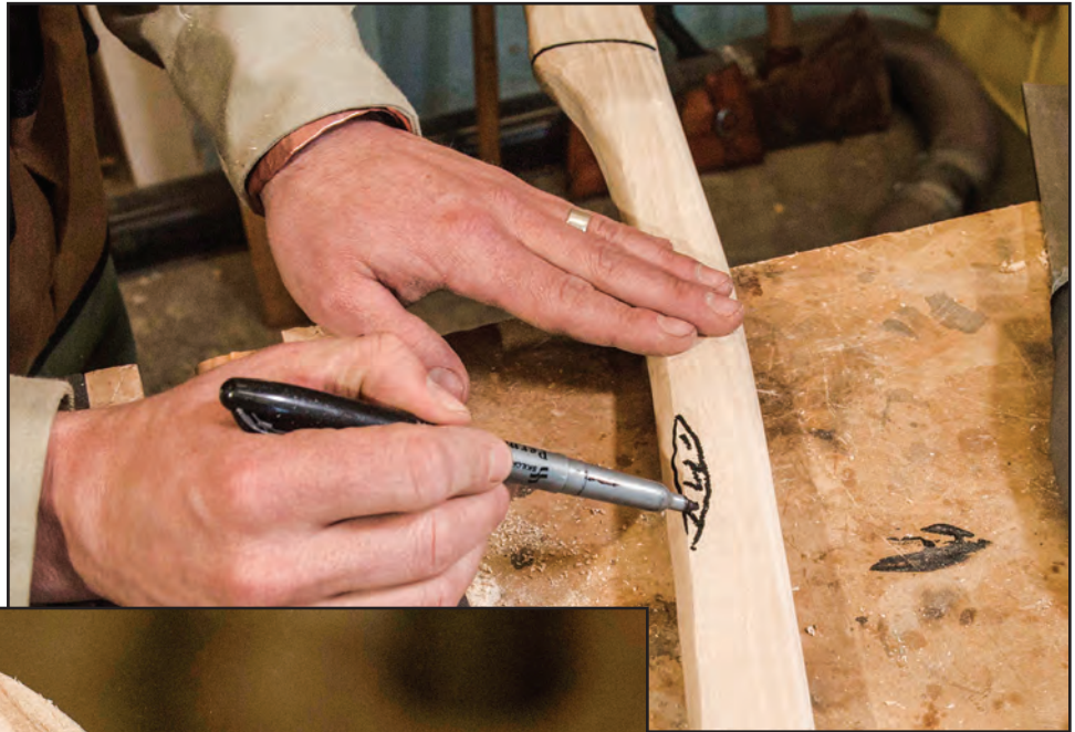
Figure 9–8—Using a felt pen to mark an ax handle.
