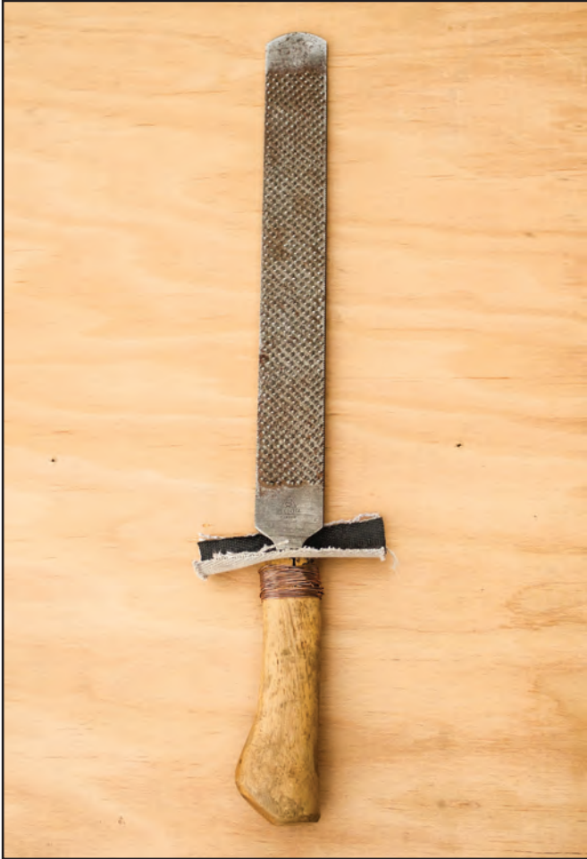
Figure 7–4—A rasp (the author used a broken ax handle to make a handle for this rasp).
