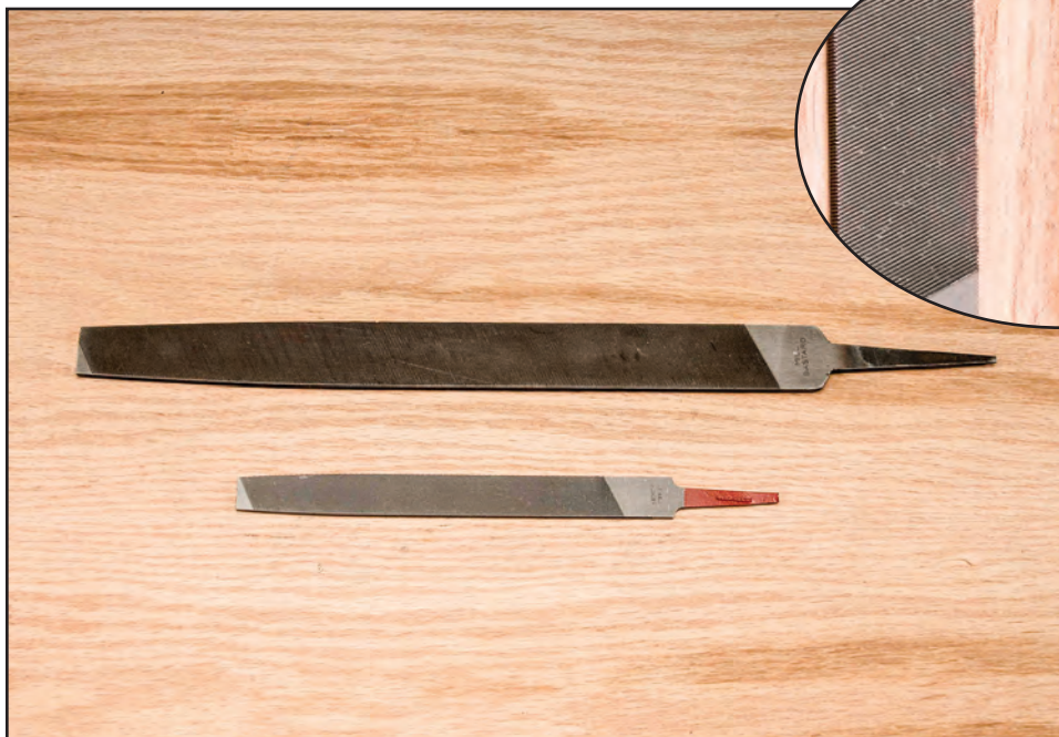
Figure 7-1—A 12-inch flat bastard file and a 6-inch flat bastard file. Note the difference in coarseness between the two files (inset).
