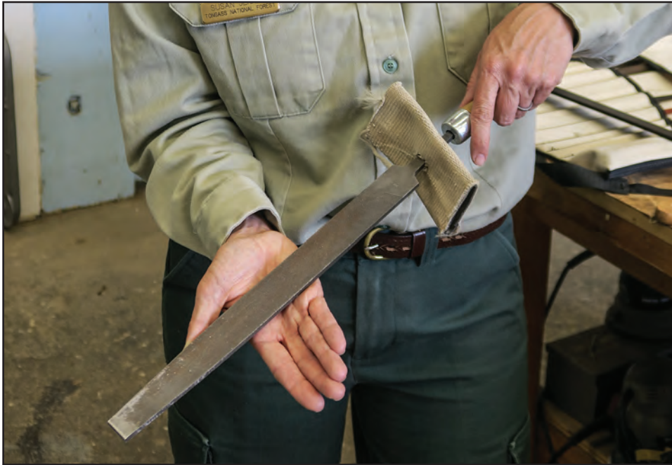
Figure 7-13—A file with a firehose handguard.
