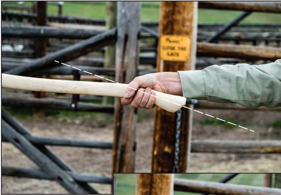
Figure 6–23—The angle of the wrist when using a curved handle (left) and a straight handle (below).
