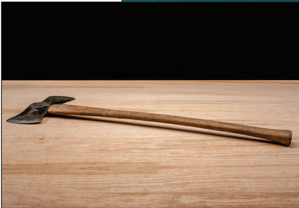
Figure 6–20—A bowed ax handle.
