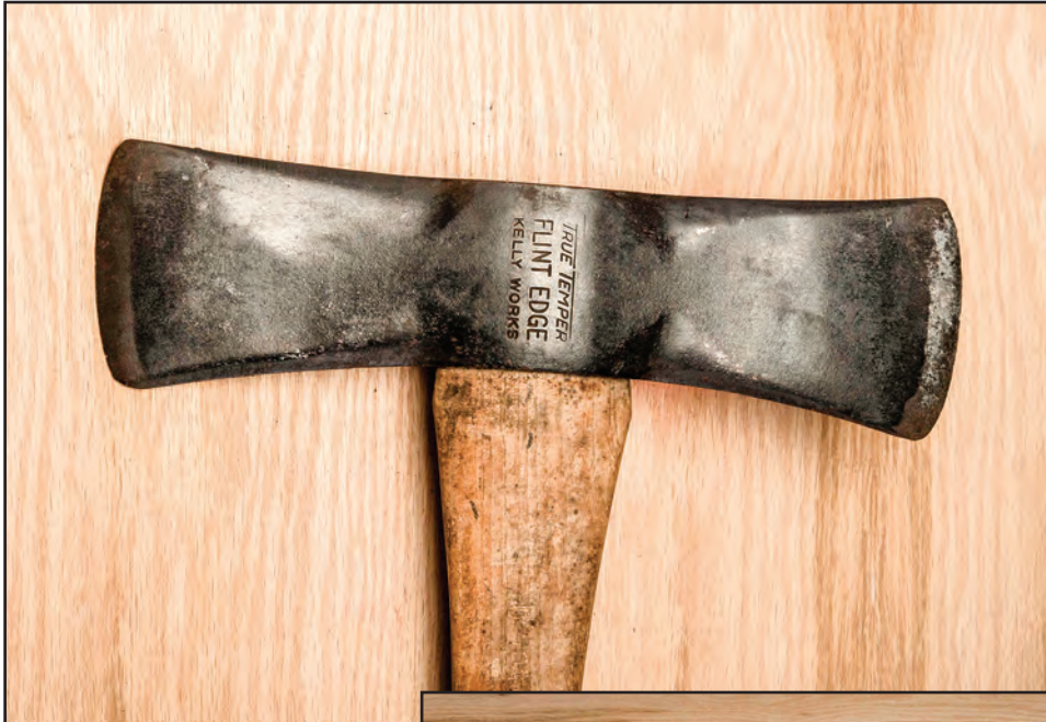
Figure 6–8—A True Temper Kelly Works Puget Sound felling ax.
