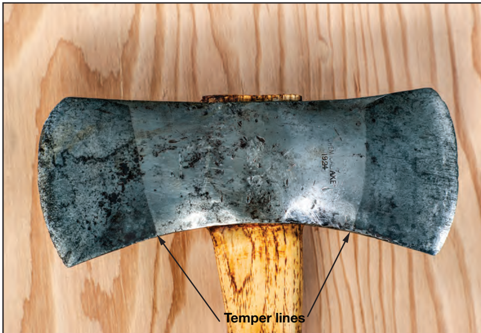
Figure 6–11—A 1924 Sager Chemical ax head with the temper lines of the blade indicated. The tempered steel is harder than the softer center of the ax head.
