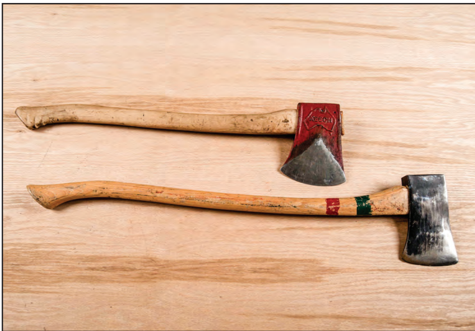
Figure 6–7—An Australian Keech ax (top) and a standard American single-bit ax (bottom). The Keech ax has a heavier head and shorter handle that is more appropriate for an experienced axman.
