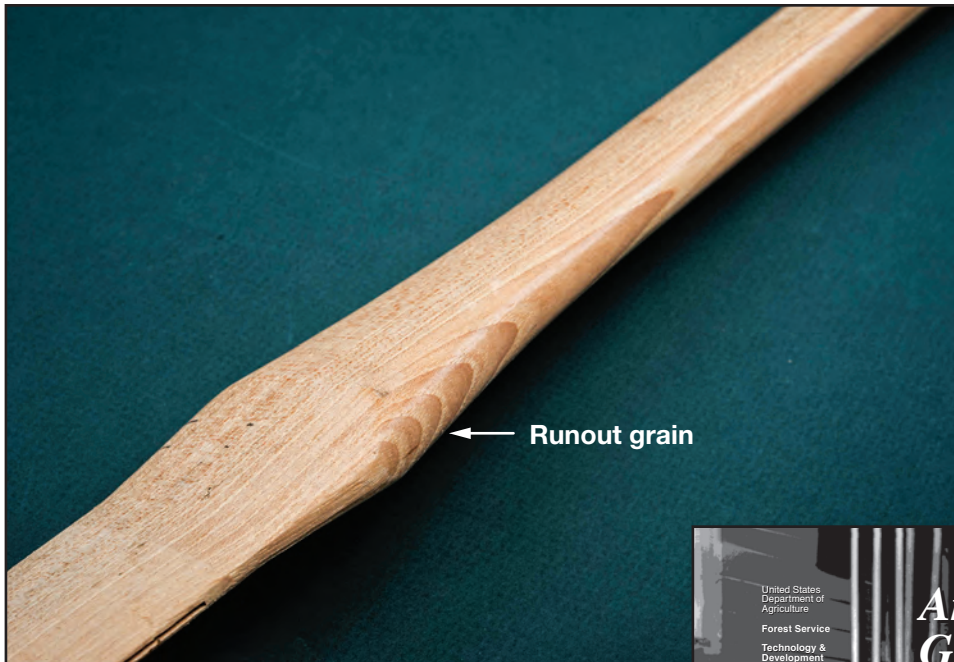
Figure 6–17—Runout grain on the back or belly of an ax handle is a sure sign that the grain runs the wrong way.
