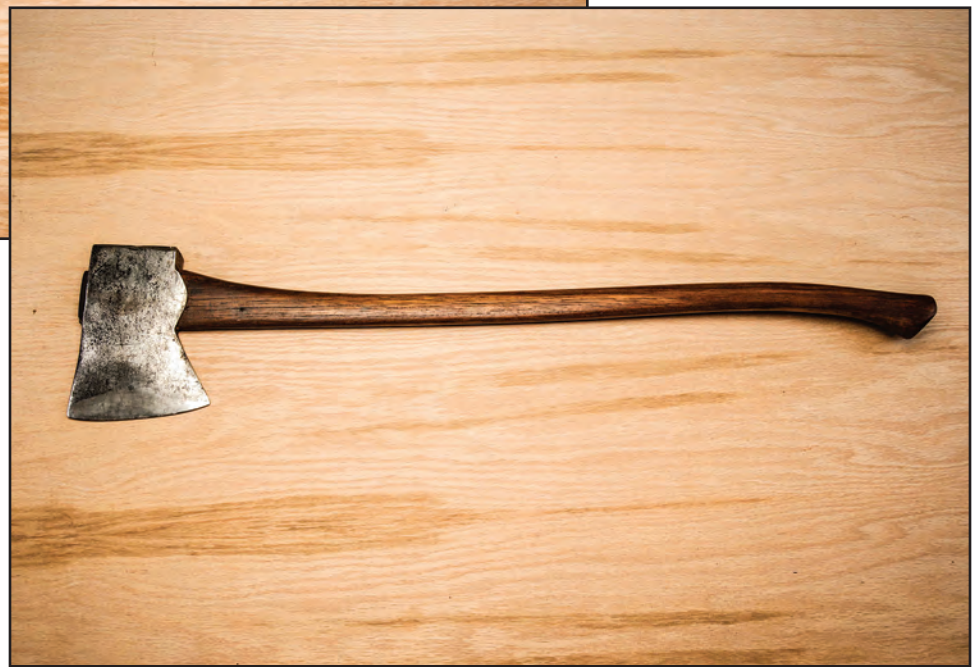
Figure 6-5—A 3½-pound Rockaway head on a 34-inch handle.
