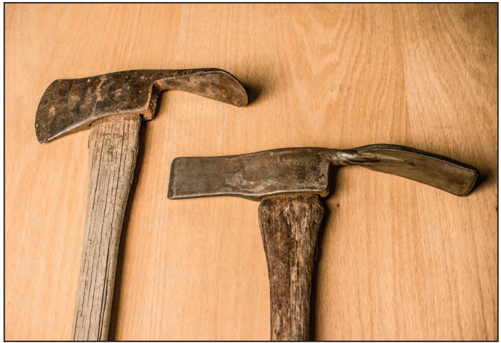
Figure 5-9—Early pulaski designs. Although designed as a wildland firefighting tool, early pulaskis were originally sold as grubbing tools.
