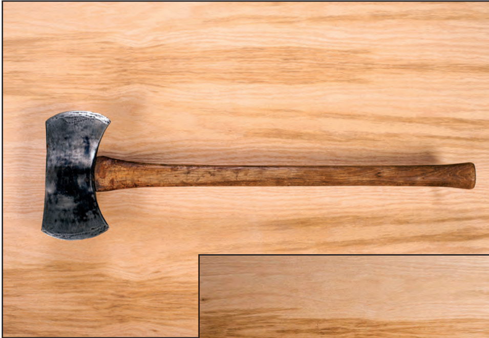
Figure 5–16—This Collins cruiser ax with a 2¼-pound head on a 28-inch handle is well suited for light-duty chopping.
