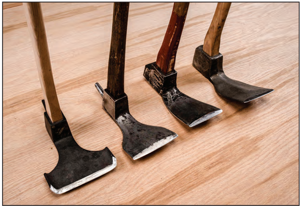
Figure 5-26—Various adzes (right)—note the differences in curvature of each blade—and a gutter adz and bowl adz (below).
