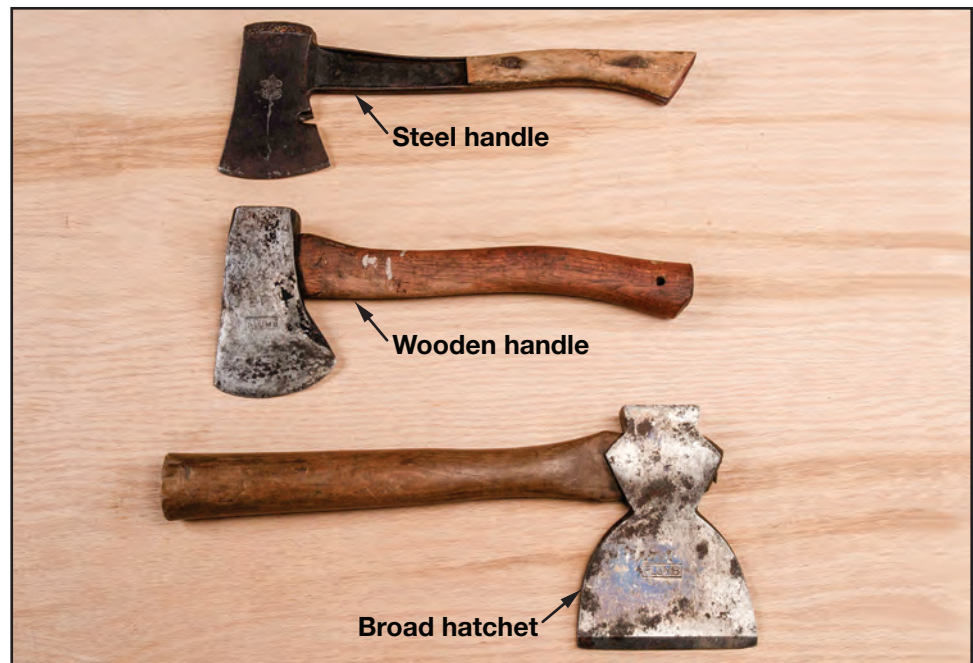
Figure 5–21 — Two Boy Scout hatchets; a Bridgeport with a steel handle (top) and a Plumb with a wooden handle (middle); and a broad hatchet (bottom). The broad hatchet, like the broadax, is used for shaping rather than general-purpose chopping.
