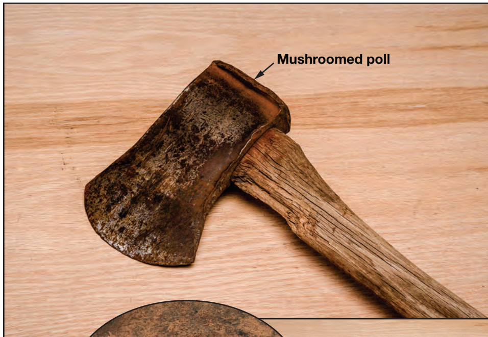
Figure 5-2—A Winchester ax with a damaged poll.
