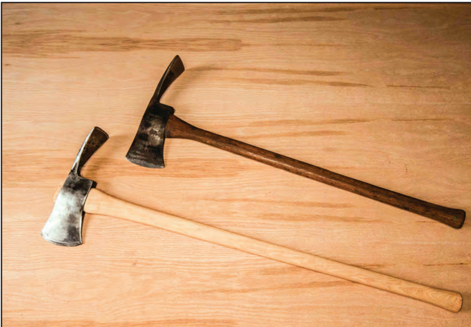
Figure 5-10—A standard pulaski with a 36-inch handle (top) and a pulaski with a 44-inch handle (bottom).
