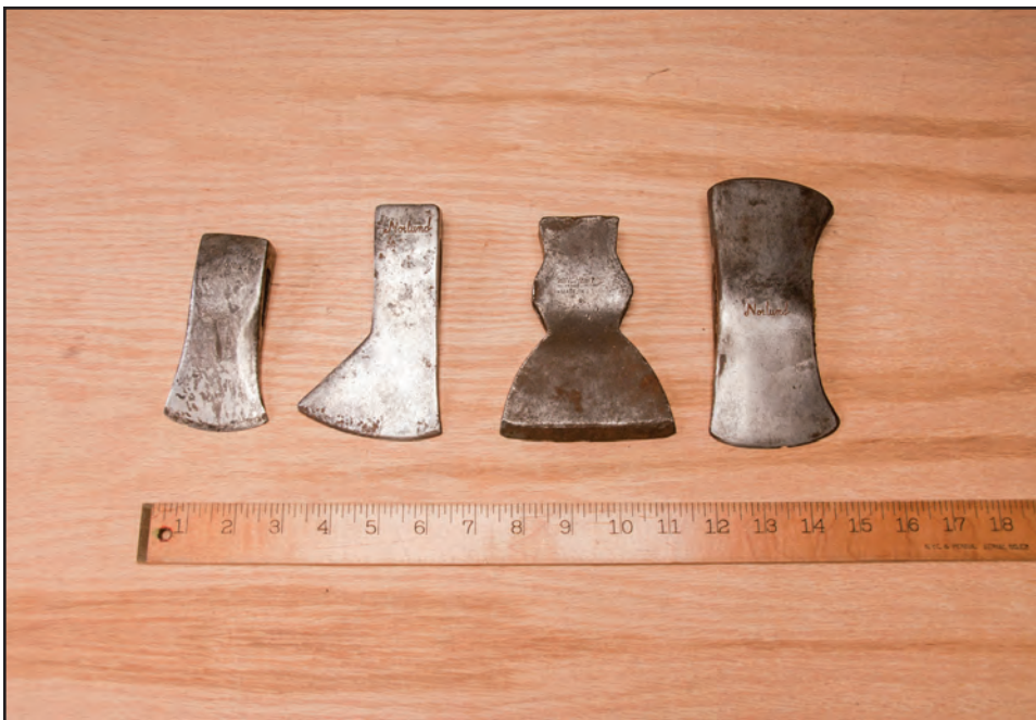
Figure 5–22—Miniature ax heads, from left to right: a single-bit ax head marked “Missoula, Mont.,” a Norlund Hudson Bay pattern single-bit ax head, a Winchester broad hatchet head, and a Norlund double-bit ax head.
