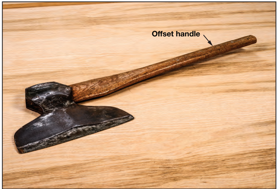
Figure 5-23—A side view of a broadax showing the offset handle.
