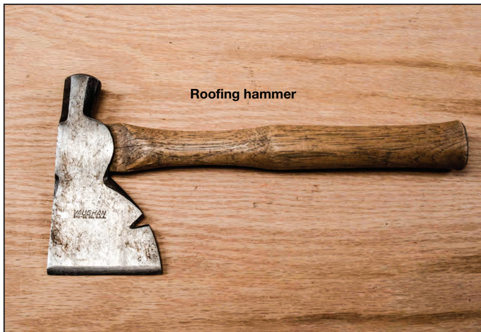
Figure 5–28—A roofing hammer (right), a fro and mallet (below), a slick (following page, top), and drawknife (following page, bottom).
