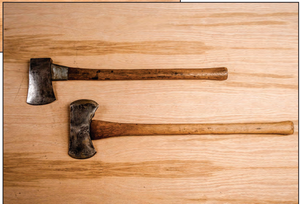
Figure 5–17—A Dillon Camp single-bit camp ax and a Marbles double-bit camp ax. Both axes have 2-pound heads.
