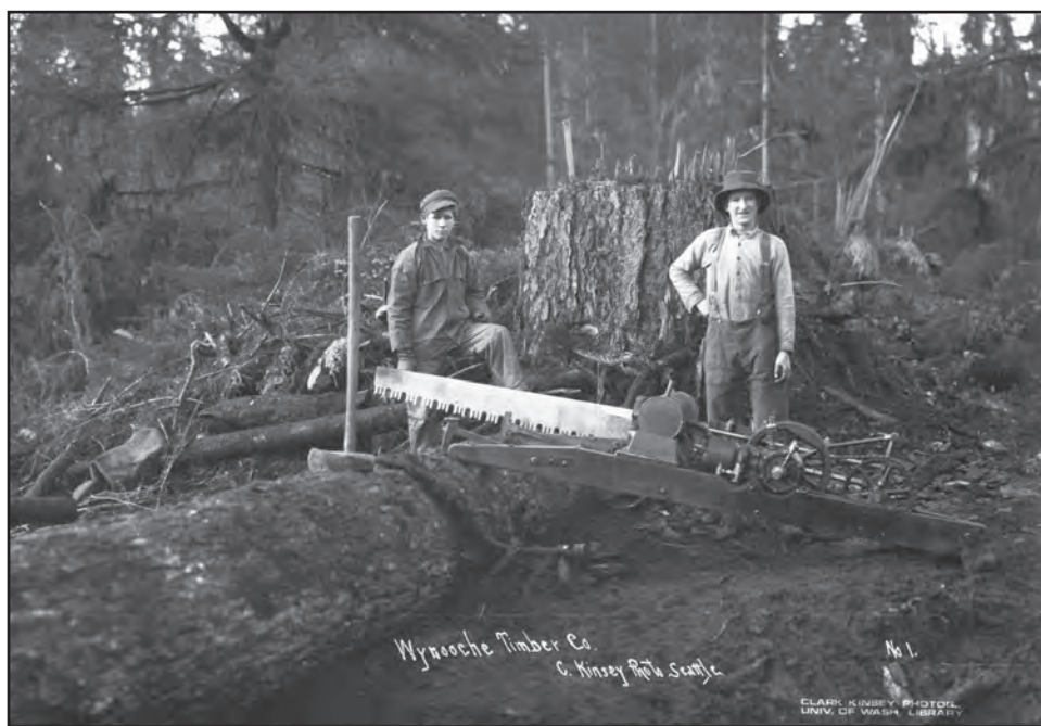
Figure 3-5—Two young loggers using a Vaughn drag saw, circa 1921. —University of Washington
