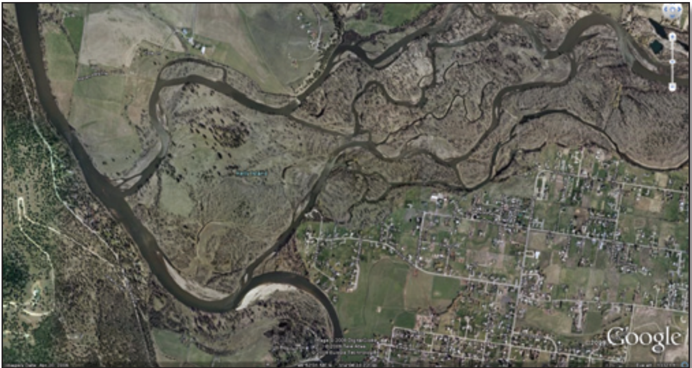
Figure 3—A series of aerial photographs taken during different years can help show whether the stream is stable at a proposed bridge site. This photograph shows the portion of Missoula, MT, displayed in the topographic map (figure 2).
