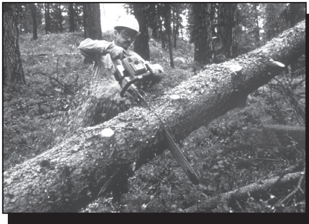
Figure 4-2—The top side of suspended logs should be limbed while you are standing on the ground or you can buck the log to lower it to the ground before limbing.
