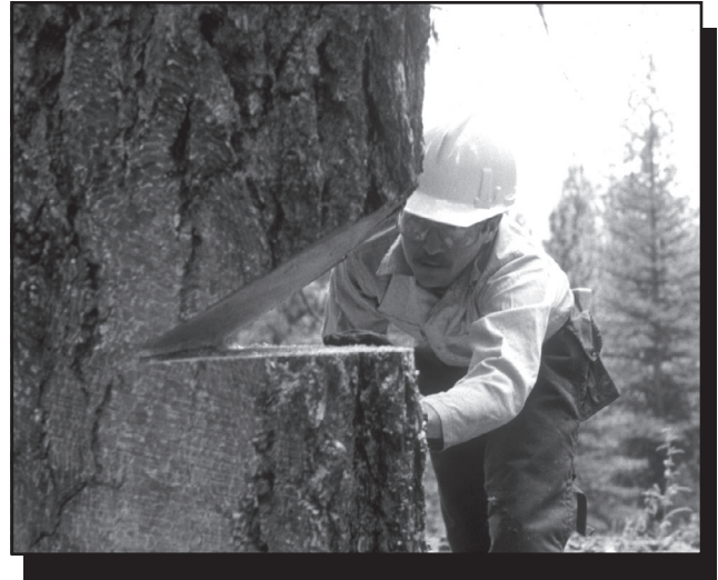
Figure 4-23—The sloping cut is a 45-degree angle.
