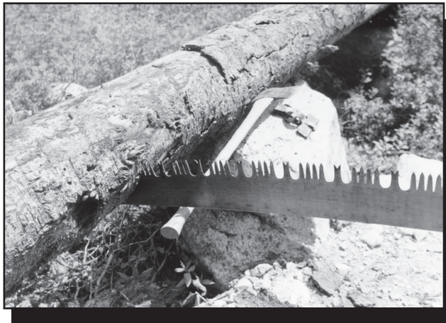
Figure 5-23—An ax planted in the lower part of the log can work as an underbuck.
