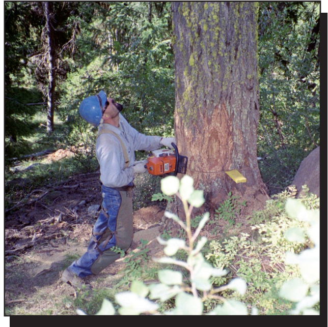
Figure 4-19—Complete the back cut.
