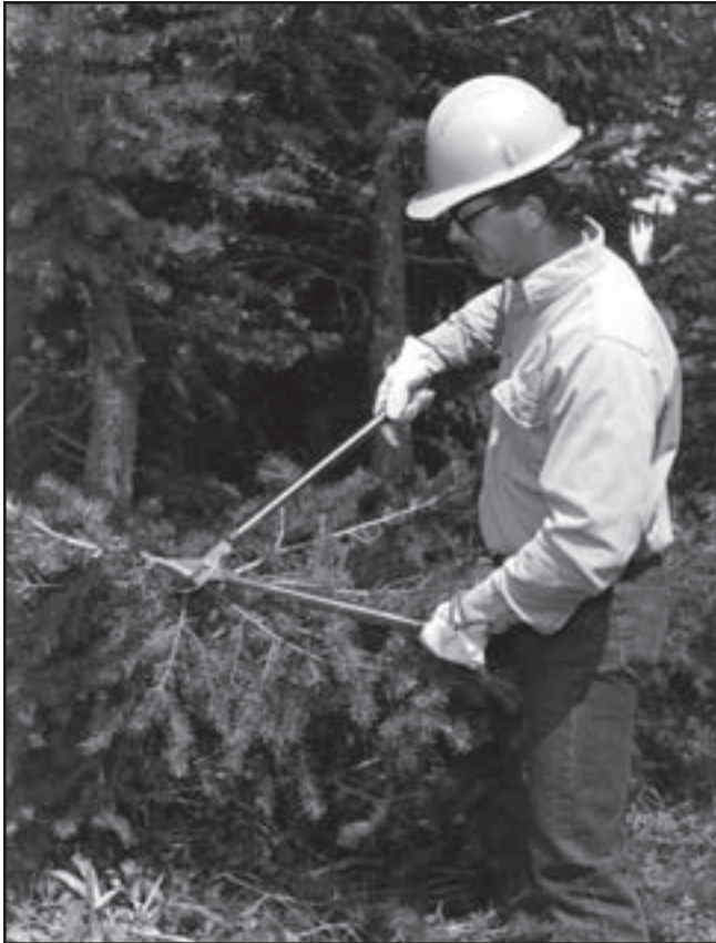
Lopping shears allow branches to be cut cleanly and flush with tree trunks.
