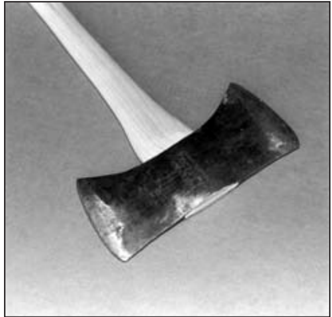
H —The finished mounted tool. The handle can be finish-sanded and oiled with raw linseed oil to protect against moisture.
