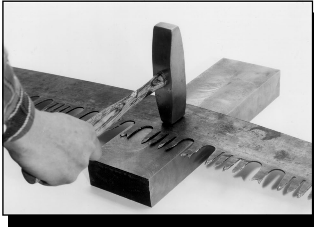
Figure 20—Hammering out a kink using a specially shaped saw hammer.
