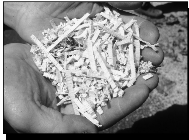
Figure 10—Long, clean shavings like these indicate a well-sharpened saw. In some parts of the country these shavings are called noodles .
