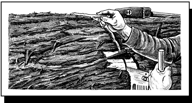
Figure 51—A stick dropped into the kerf on a log with bottom bind will serve as a pivot when the log is cut through. This is a lost trick that is very practical and can prevent damage to the saw.— Now You're Logging , by Bus Griffiths, with permission of Harbour Publishing, Madeira Park, BC, Canada
