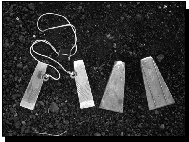
Figure 38—Wedges made from soft metals such as magnesium and aluminum are stronger than plastic, can be used as hanging wedges, and will not damage the saw.
