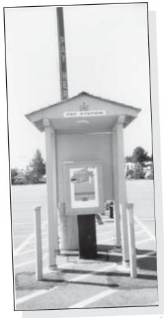
Figure 10—A tall sign allows boaters to spot the VenTek System 5 Pay Station in the parking lot even when the lot is full. Metal pipe protects the shelter and machine from vehicles.
