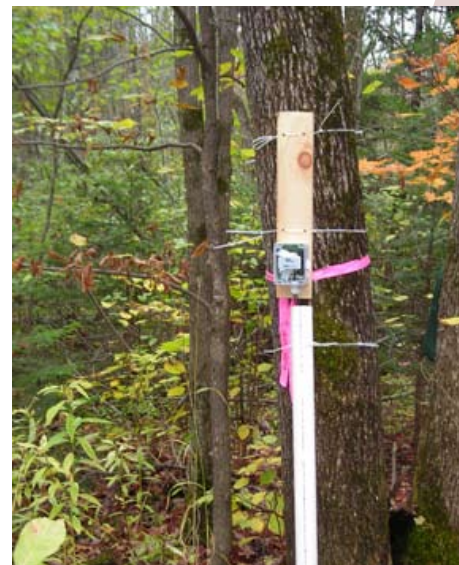
Hobo datalogger attached to tree. Datalogger will record soil moisture and soil and air temperature throughout the winter.
