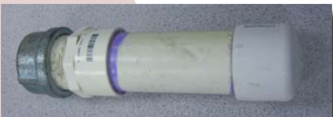
Figure 6. Winter log 2 - PVC pipe with soil temperature probe is buried within the unit to determine soil temperature.
