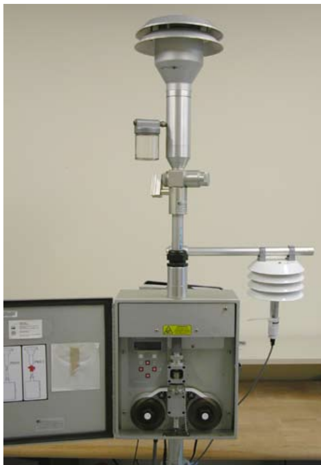
Figure 11. The E-BAM smoke particulate monitor.
