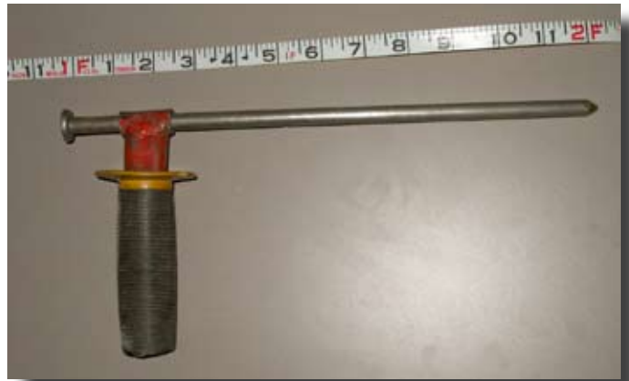
Figure 7. Winter log 3 - Simple tool to measure depth of frozen soil (Hiawatha NF).
