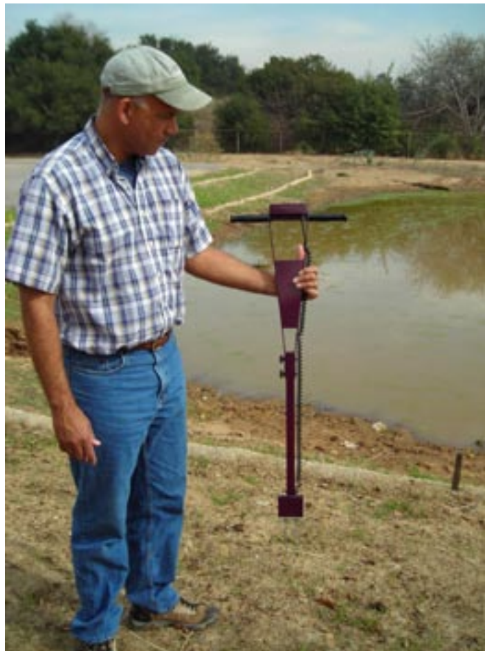
The Field Scout TDR is one of the soil moisture devices being evaluated.
