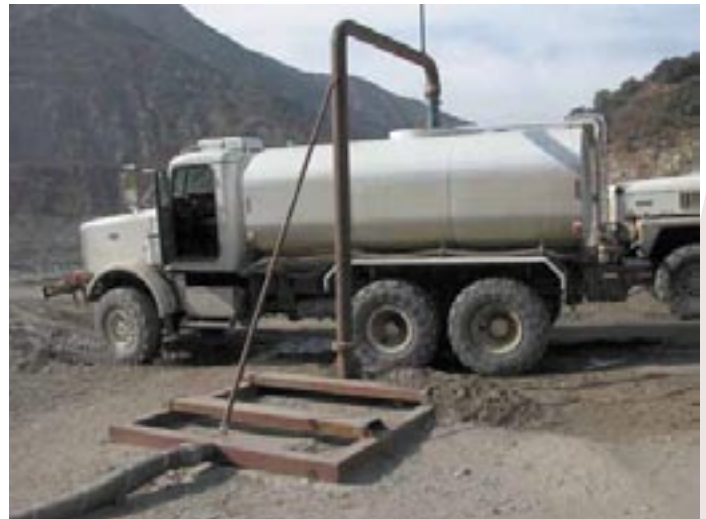
Figure 6—Standpipe used to fill water truck.
