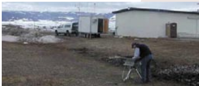
Figure 2—Andy Trent adjusts the SODAR antennae at the Granby, CO, airport. The white trailer houses the SODAR electronics, satellite communications, and instruments to measure surface weather, ozone, and oxides of nitrogen.
