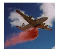
**Multi-engine Airtanker:** A fixed-wing aircraft with more than one engine certified by the FAA as being capable of aerial delivery of fire fighting chemicals. Most multi-engine airtankers have a 1800- to 3000-gallon capacity.
