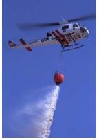
**Helibucket:** A specially designed bucket carried by a helicopter, like a sling load, and used for aerial delivery of fire-fighting chemicals including water. The bucket can be quickly detached so that the helicopter can be used for other assignments.
