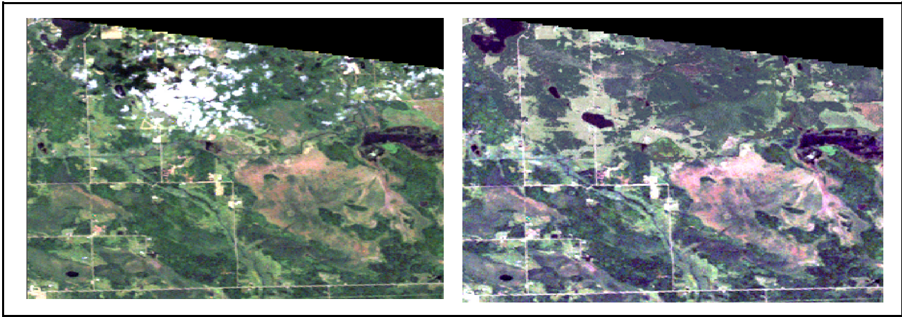
Figure 5—Above left, the original Landsat EMT+ image with clouds; above right, the EMT+ image with the clouds removed by using the eliminate clouds procedure developed at RSAC.
