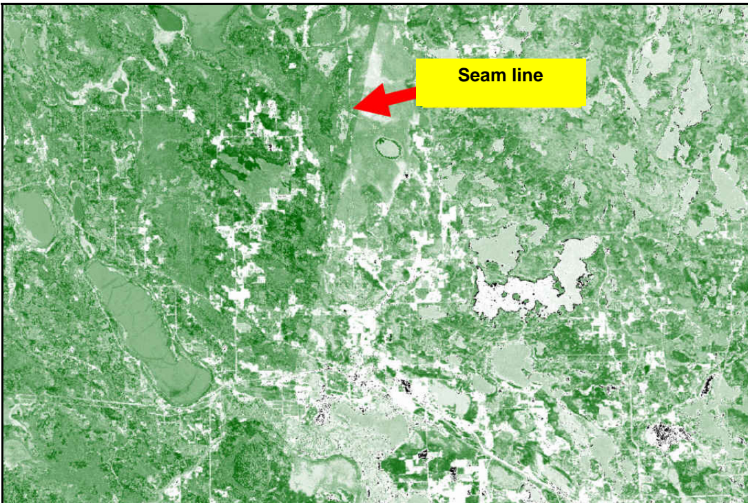
Figure 7—Examples of bad results obtained for the canopy-cover layer of Zone 41. These artifacts of modeling were eliminated using the highlighted model shown in table 3.
