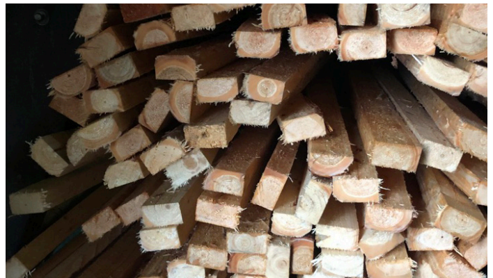
Small diameter timber lamstock sawn at the F.H. Stoltze Land and Lumber sawmill. Courtesy of Wooden Haus Supply.
