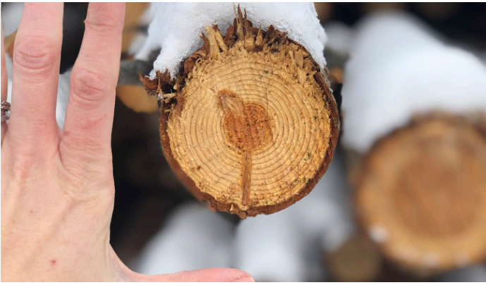
A small-diameter log, harvested from a national forest, that will be used to make cross-laminated timber. Courtesy of Wooden Haus Supply.
