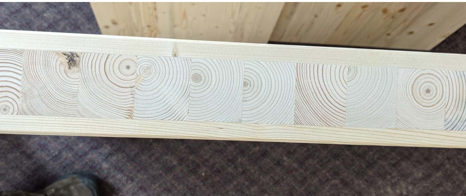
Cross-laminated timber panel made from small-diameter logs harvested from a national forest. Courtesy of Wooden Haus Supply.
