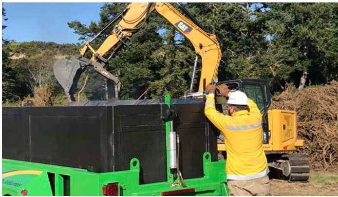
This biochar production unit and loader are an example of moderate-scale biochar production using an invasive woody plant called gorse. USDA Forest Service photo.
