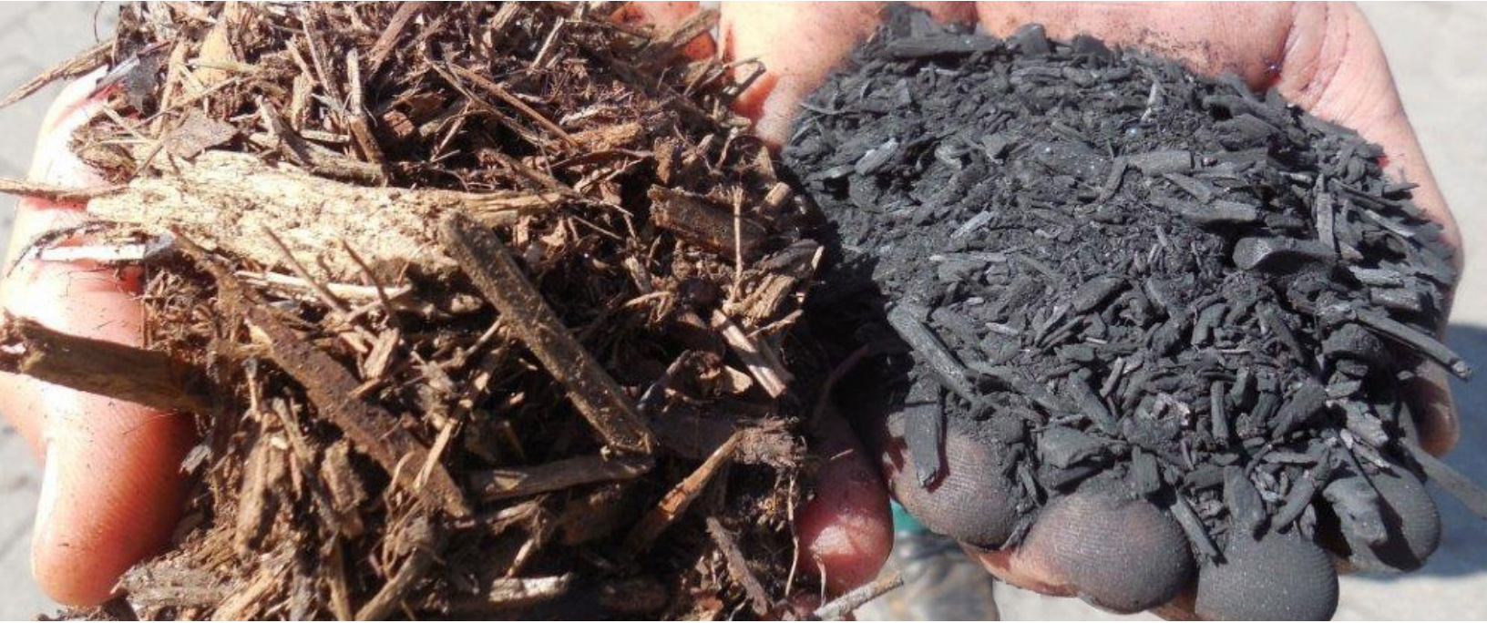
Biochar (right) is the carbon-rich solid produced by heating biomass (left) under low-oxygen conditions. Courtesy photo by Biomacon.
