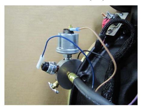
Attach manifold to engine flywheel housing, circuit breaker may have to be moved. Attach ground wire with manifold.
