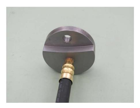
Attach hose to manifold 4228300, NPT thread, before mounting to engine.
