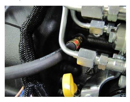
Install hose part number 4430920. NOTE: The hose has BSP threads and NPT threads, the hose end with BSP threads fits the engine block.
