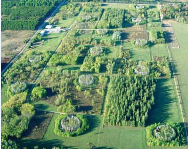
Figure 3. Infrastructure needs to study climate change impacts: FACE (Free Air CO 2 Enrichment) experiment conducted at Forest Service Northern Research Station facilities in Rhinelander, WI. CO 2 is pumped out of pipes, controlled by sensitive anemometers, in order to assure a high CO 2 concentration at all times inside each ring. The photo shows several replicates of experimental (CO 2 , ozone) fumigations, and the control rings (no fumigations). FACE experiments require $1 to 2 million in CO 2 supplies and maintenance, yearly. Photo by David Karnosky, Michigan Technological University.
