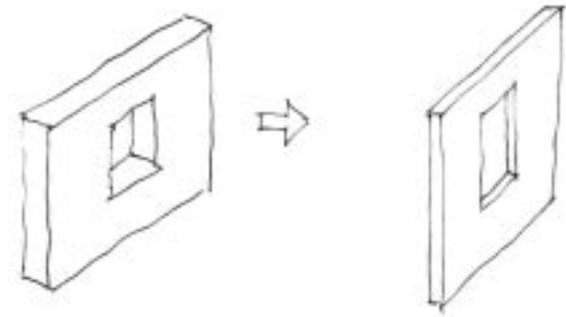
**Walls should be thinner in California mountains due to more temperate climate and greater seismic activity**
