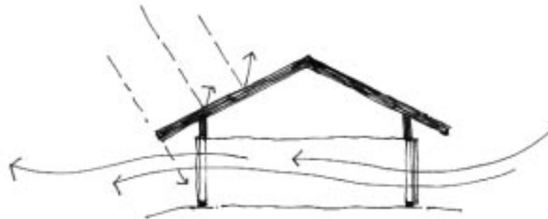
Natural ventilation and shading are maximized
