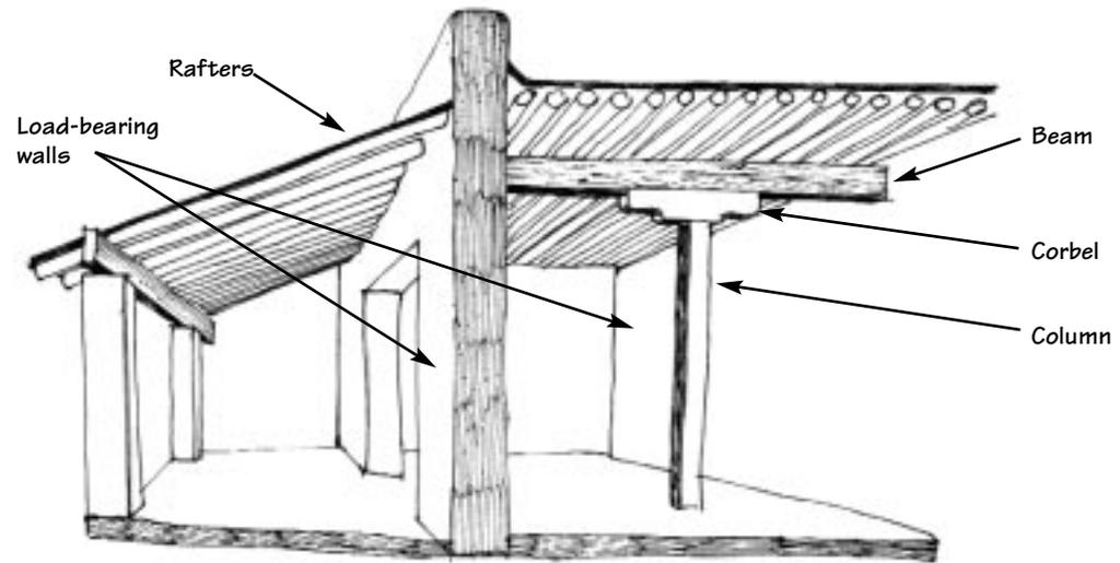
Exposed structure should be limited primarily to roof supports
