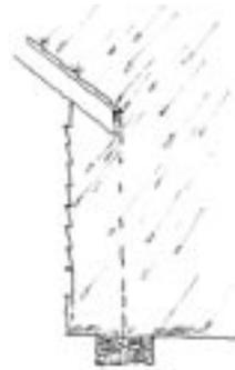
Roofing extended to accommodate dripline
