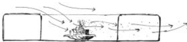
Courtyard with water feature for evaporative cooling
