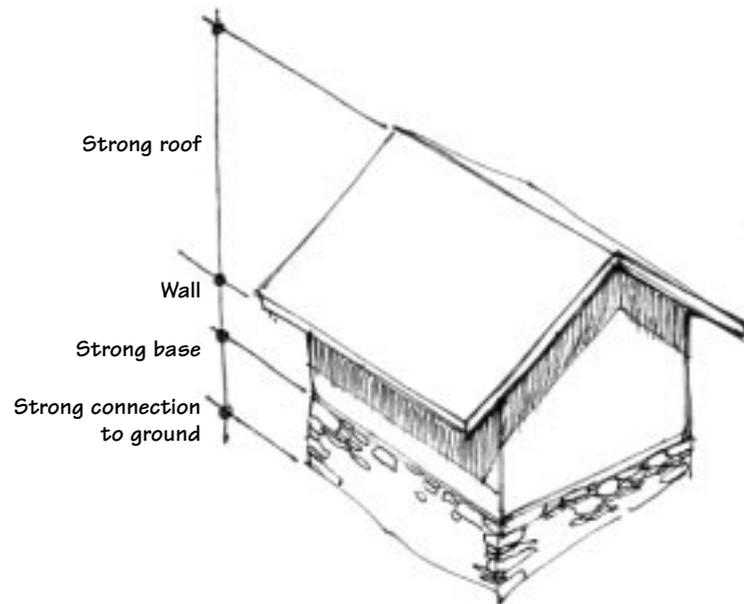
Wall is subservient to roof and base
