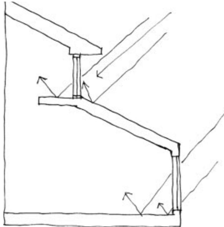
Daylighting should be maximized by adding high windows for additional daylighting
