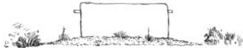
**Selectively clear vegetation & slope away from structure for drainage**
