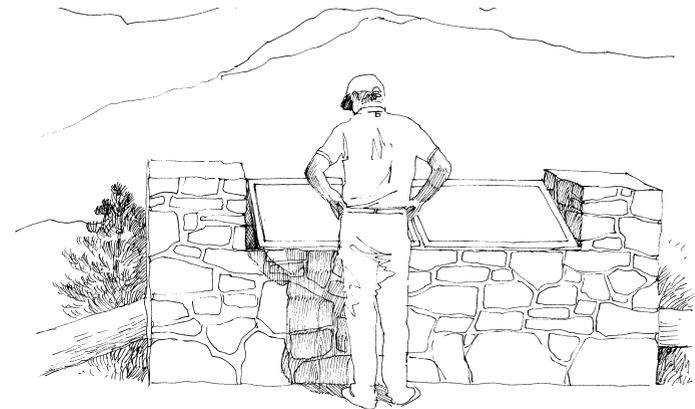
The low-angled mounting of this interpretive sign does not block the view and reduces sun glare
