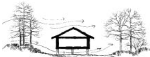
Ground cover cleared and structure raised for ventilation
