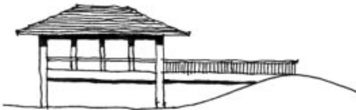
Access to raised level utilizing grade and boardwalk
