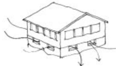
Lower structure in cooler climate, retaining ventilation
