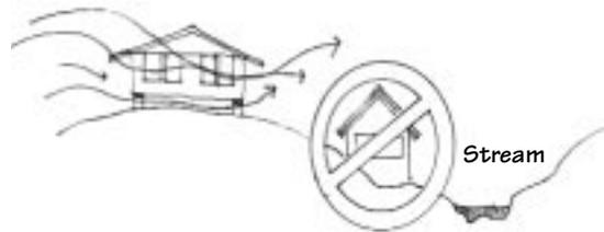
Structure placed well above and away from stream to avoid flooding and insects
