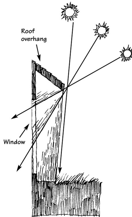
Length and placement of a fixed roof overhang determines amount of natural light entering a building at different seasons or times of day
