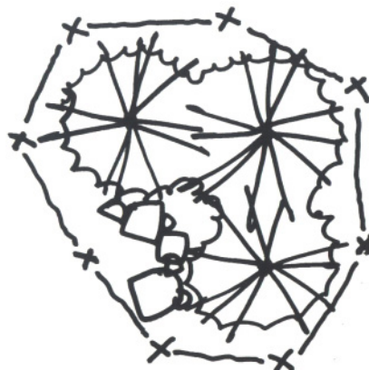
Fence around healthy trees/shrubs to protect them from construction activities
