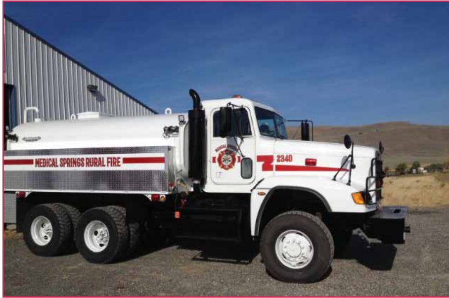
Figure 2 —A water tender converted from a military truck tractor through a Federal surplus equipment program. Photo: Oregon Department of Forestry.
