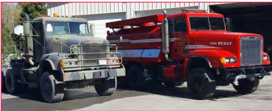
Figure 4 —An original military Freightliner Truck Tractor next to a truck modified as a water tender. Photo: Oregon Department of Forestry.
