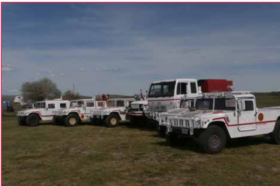
Figure 5 —Fleet of the Silver Creek Rangeland Fire Association, with Humvees converted into type 6 engines and a cargo truck converted into a water tender. Photo: Oregon Department of Forestry.
