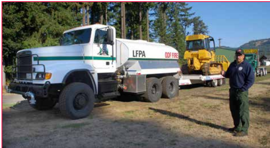
Figure 3 —With a smaller water tank, a modified surplus military truck can pull a dozer. Photo: Oregon Department of Forestry.
