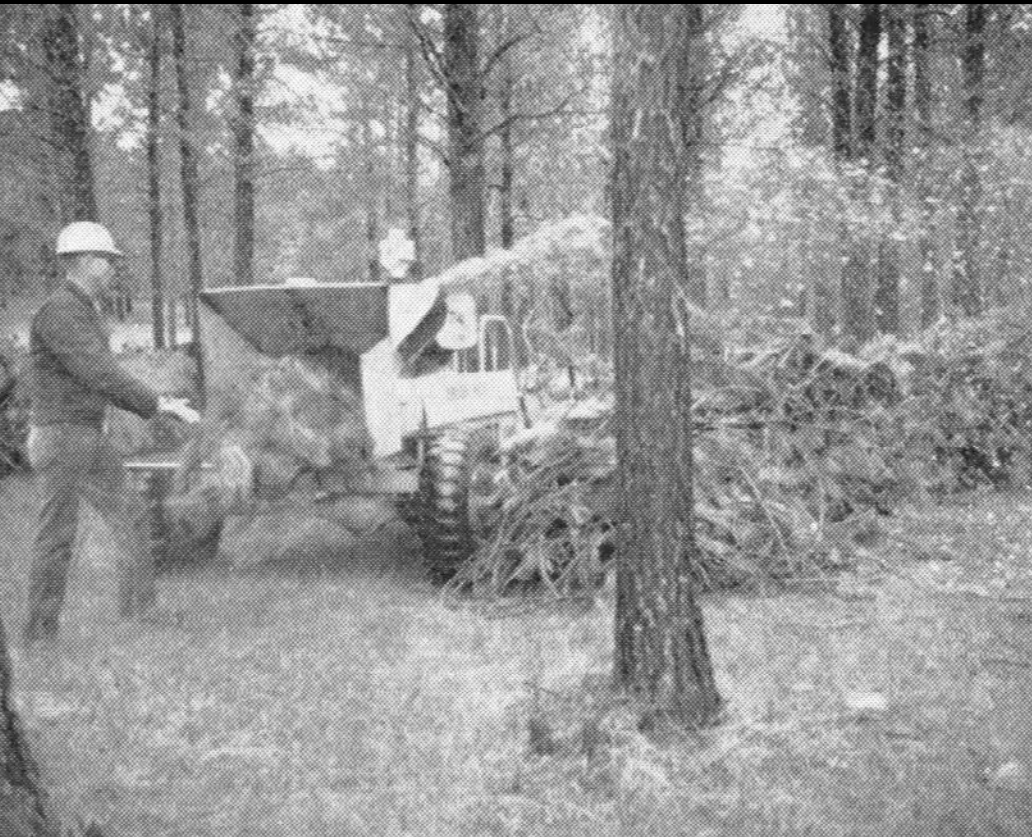
Figure 1 —This self-propelled chipper is being used on windrowed brush piles.
