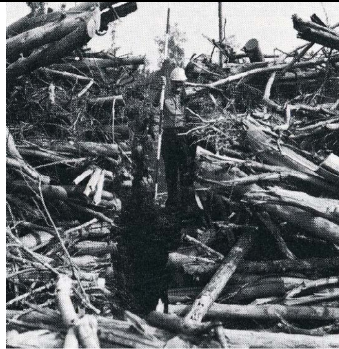
Figure 4 —Material from a transverse 2-foot (0.6-m) section of the windrow was removed, separated into size classes, and weighed.
