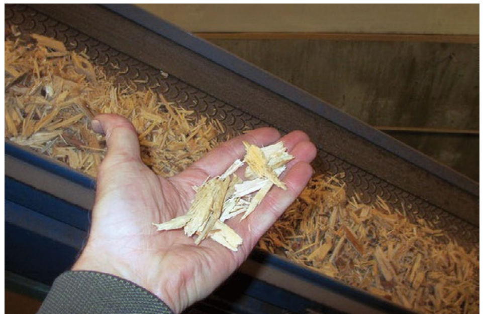
Wood chips fuel the boiler for a school in Alaska. USDA Forest Service photo.
