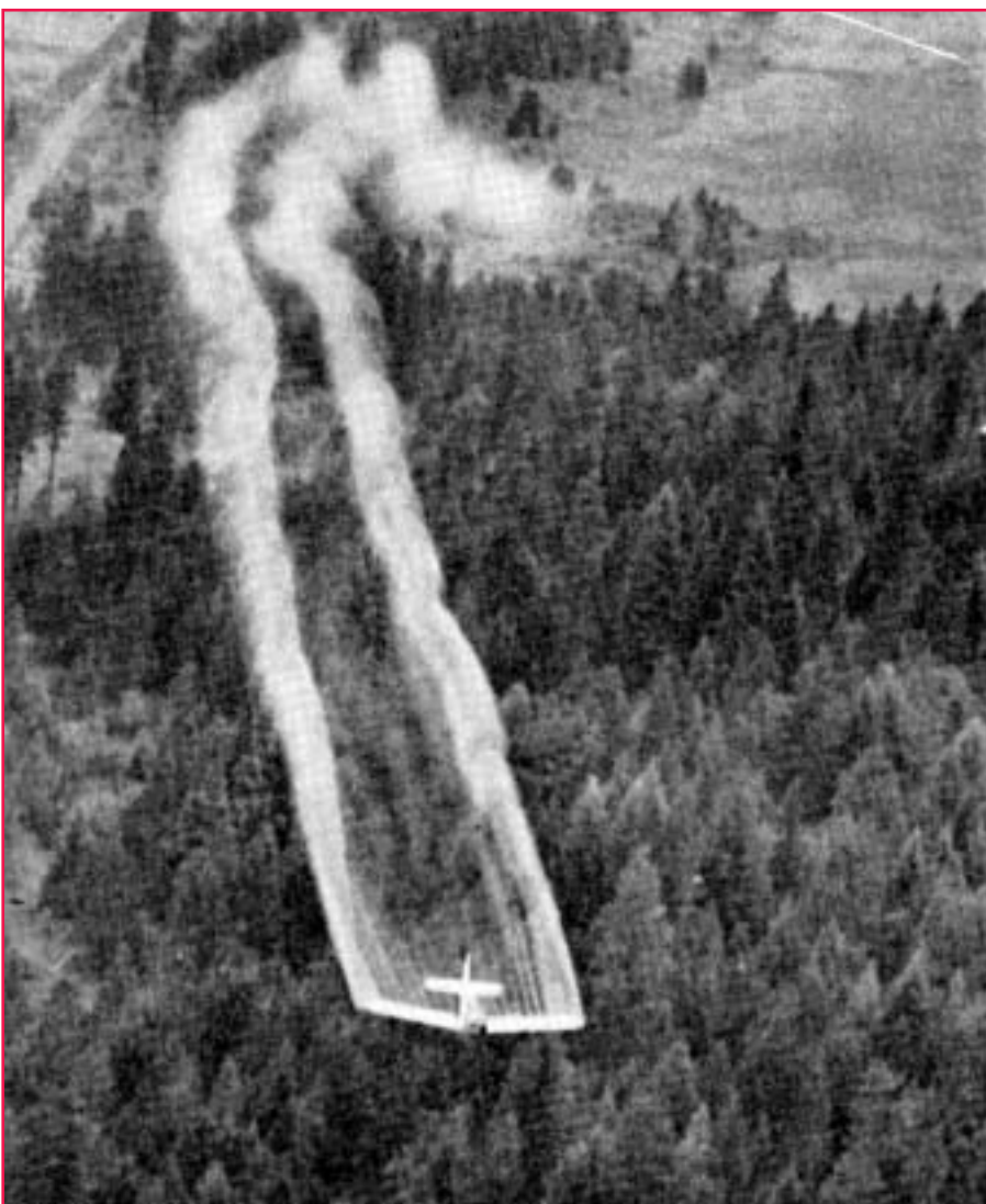
Figure 1 —Low-flying spray plane. Note funneling effect of spray trailing behind each wingtip. This is vortex turbulence.
