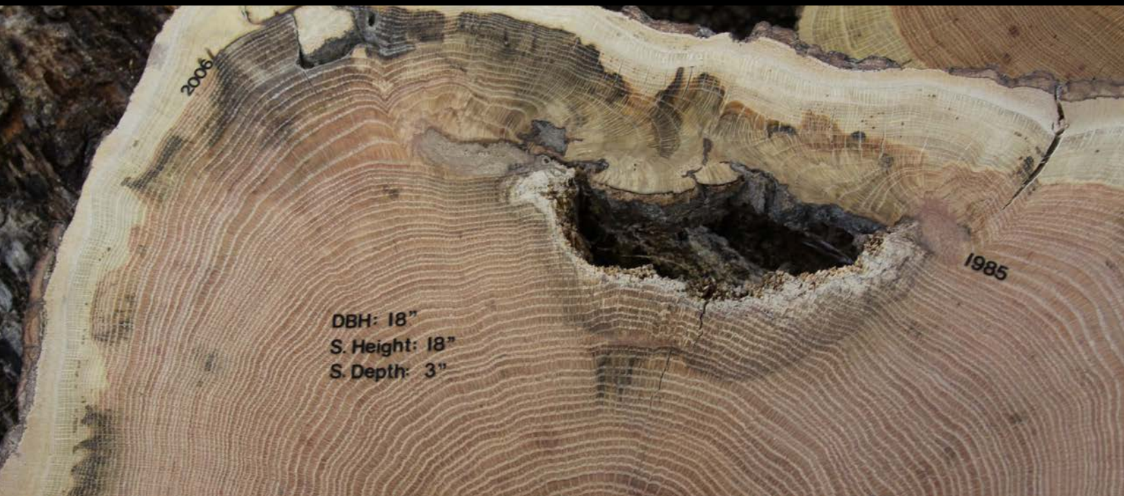
Figure 5 —This mature white oak was wounded by fire in a northern Missouri woodland but was able to compartmentalize the fire injury, close over the open wound, and thereby minimize wood loss to decay. Some mineral stain has formed in reaction to the injury and infection, which degrades lumber value. Since fire injuries occur on the large end of the butt log, any damage remains outside of the scaling cylinder for a time and hence has minimal impact on log and lumber value. Harvesting injured trees within 5 to 10 years after injury also minimizes volume and value loss. Photo: Dan Dey, USDA Forest Service, Northern Research Station.
