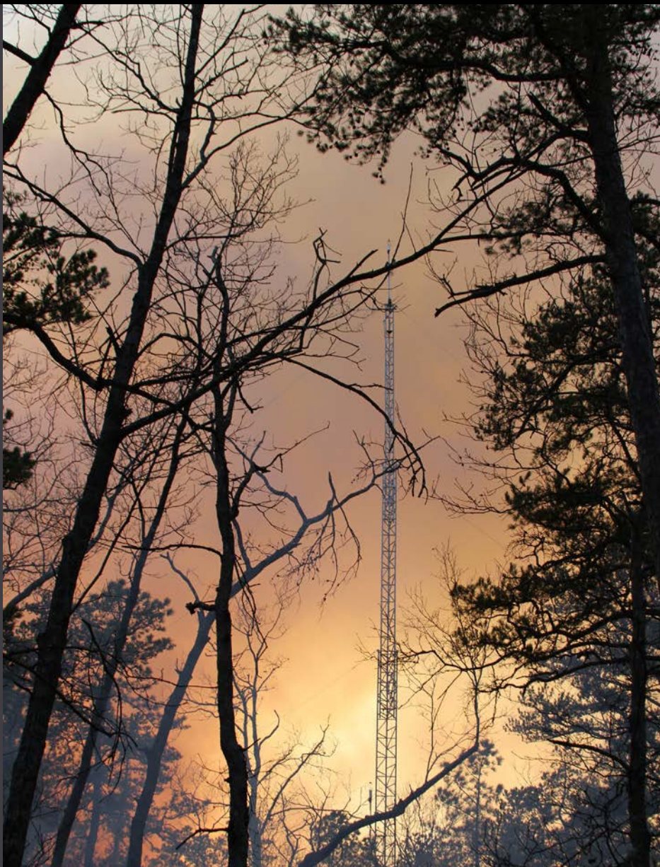
Figure 1 —Instrumented 30-meter (98-foot) mobile tower set up in the interior of a burn block in the New Jersey Pinelands National Reserve in 2011 to measure atmospheric turbulent circulations at multiple heights in the vicinity of a spreading prescribed fire beneath forest overstory vegetation. Photo: Nicholas Skowronski, USDA Forest Service.
