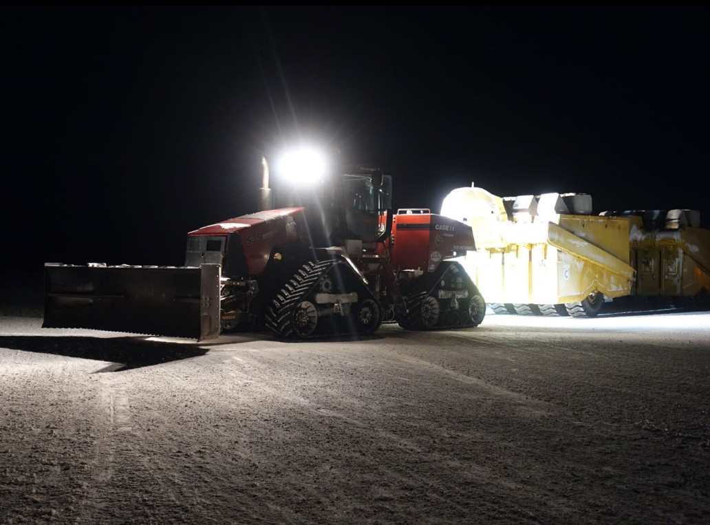
Figure 2 —A rubber-tracked tractor used as part of the U.S. Arctic Program could tow a fire tanker. It could be used on a wildfire in the wildland–urban interface both offroad and on paved roads without tearing up the asphalt. Photo: National Science Foundation, U.S. Arctic Program.
