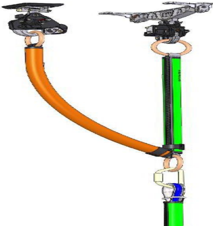
Onboard Systems Dual Hook Kit overview for Bell 206L and 407 models
