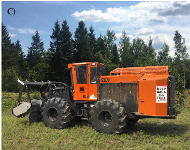
Figure 2 —A variety of carrier machines including excavators, skid steers, tractors with hydraulic attachments, and tractors with power-takeoff attachments can have attached mulching heads (photograph 2a provided by Nikia Hernandez, USDA Forest Service, Kootenai National Forest; photograph 2b provided by Mel Peterson, Director of Marketing and Training, Diamond Mowers; photograph 2c provided by Dana Mitchell, USDA Forest Service, Southern Research Station).
