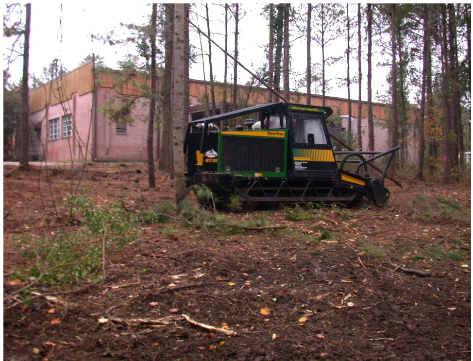
Figure 1 —Mastication machine treating surface fuels and providing a fire break surrounding buildings (photograph by Dana Mitchell, USDA Forest Service, Southern Research Station).
