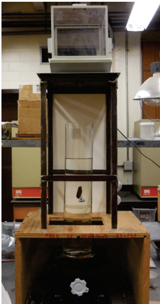
Figure B.3 —Apparatus used to estimate the density and volume of masticated fuel particles. (A) Parts of apparatus include a scale (top), a fluid column with two fluids (kerosene at top and a 50:50 mixture of glycerin and water at bottom), and a lift (bottom) to raise and lower fluid column. (B) Closeup of a particle in kerosene. Particle has weight attached to assure it stays submerged in each fluid.
