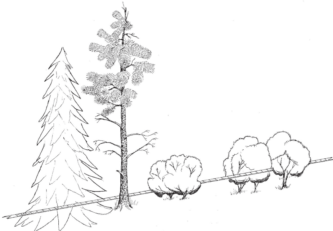
Figure LI-1 — The measuring tape is stretched taut below, in, or above the canopy vegetation, whichever position allows the easiest estimation of cover without the tape zigzagging around plants.
