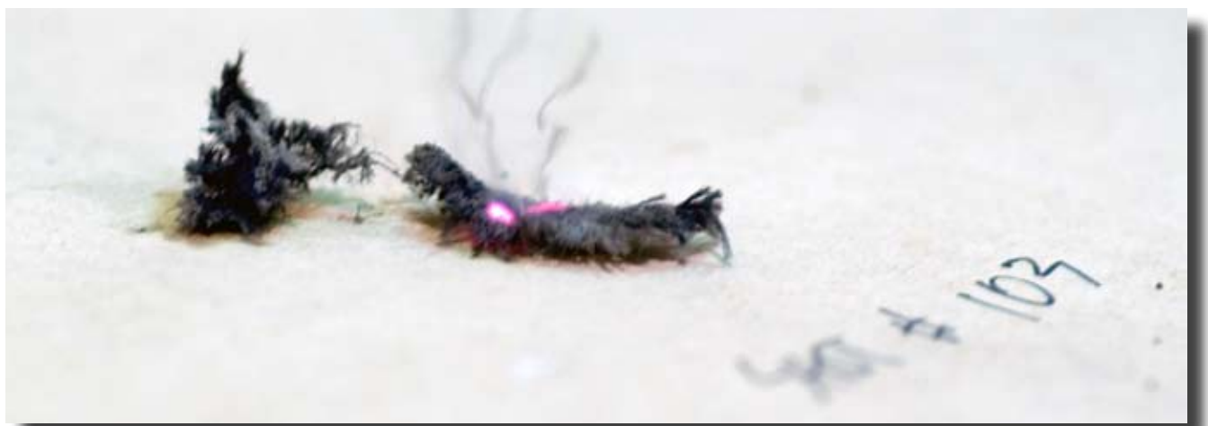
Figure 4—Smoldering patch, observation 103 (50-grain black powder, 0.010-inch-thick patch lubricated with shortening).
