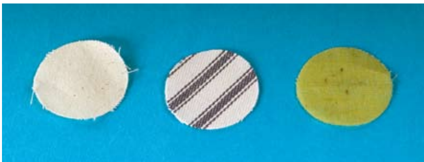
Figure 3—Patches (left-to-right): cotton (dry), pillow ticking (dry), and cotton (with commercial lube).
