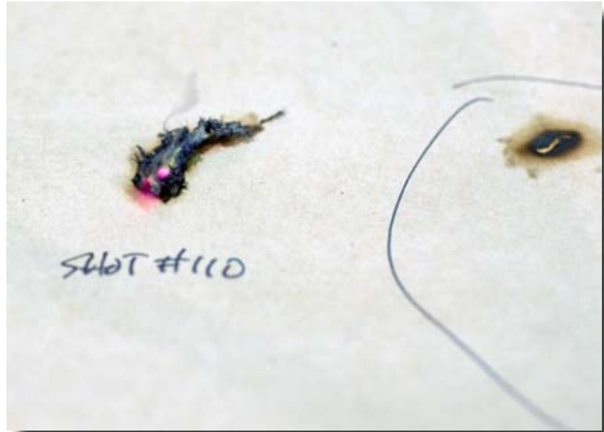
Figure 5—Smoldering patch, observation 110 (50-grain black powder, dry 0.010-inch-thick patch).
