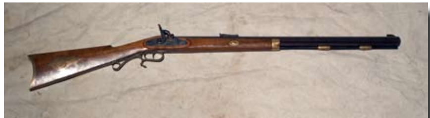
Figure 1— .50 caliber side-hammer percussion rifle (test rifle).
