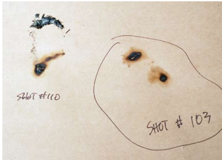
Figure 6. Positive indications of ignition on ignition receptor for observations 103 and 110.
