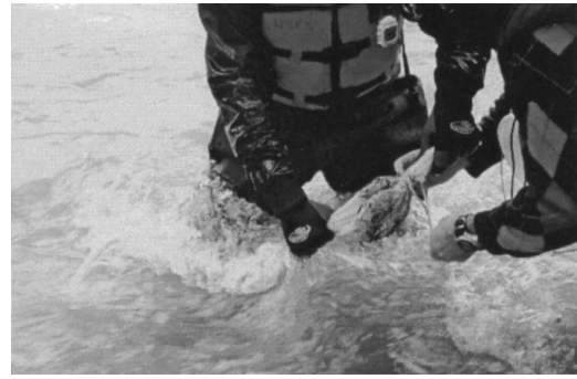
Fig. 3. Untying the net before emptying the bedload traps at Little Granite Creek
