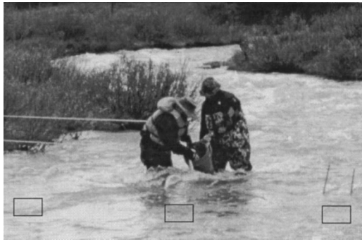
Fig. 2. Traps installed at Little Granite Creek are submerged at bank-full flow. The black rectangles indicate the location of four of the six traps (view downstream).
