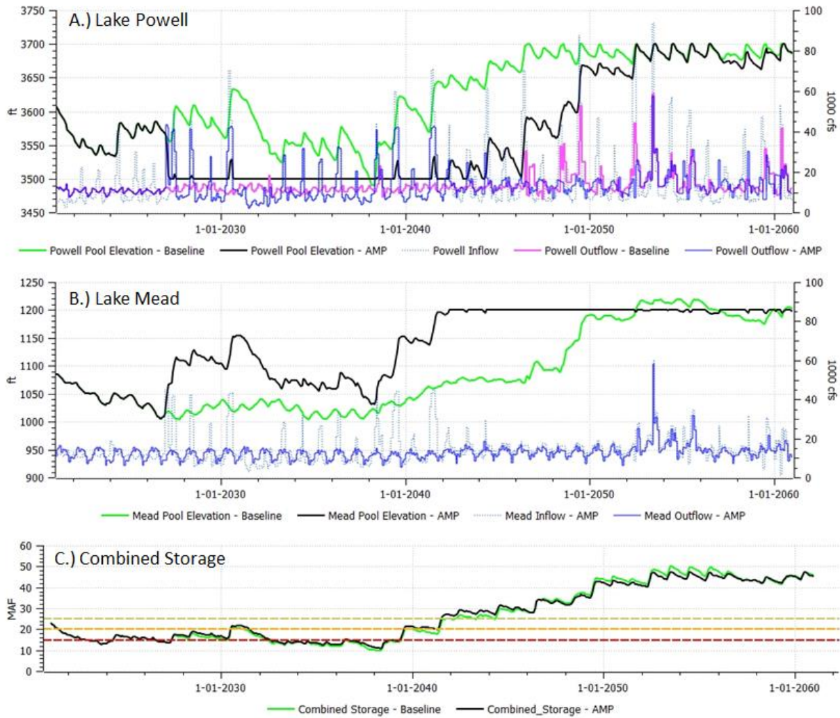
Figure 9.8. Reservoir characteristics comparing baseline and the FMF-A1 AMP with a sample Dry to Wet hydrology. (A) shows Lake Powell elevations, inflows, and outflows. (B) shows Lake Mead elevations, inflows, and outflows. (C) shows combined storages with shortage thresholds.
