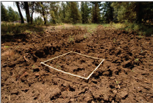
Figure 2-7—A sampling quadrat at a site with heavy equipment wheel tracks created from operating in suboptimal moisture conditions.
