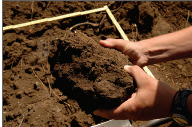
Figure 2-8—A soil clod created from the heavy equipment at the site in figure 2-7.
