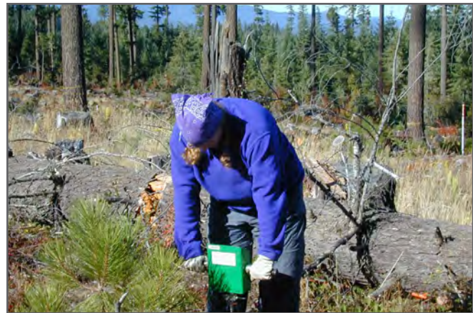
Figure 3-3—Using a one-person soil penetrometer to determine soil strength.
