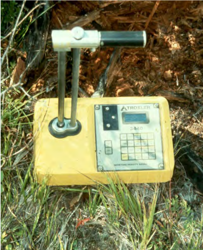
Figure 2-11 —A geophysical (neutron) soil moisture and density gauge.
