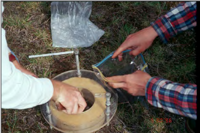
Figure 3-1—Preparing a site to determine soil bulk density using the water displacement method.
