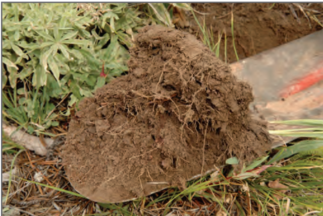
Figure 2-4—A closeup of the soil structure from the undisturbed, reference site in figure 2-3. Notice the abundance of roots throughout the sample.
