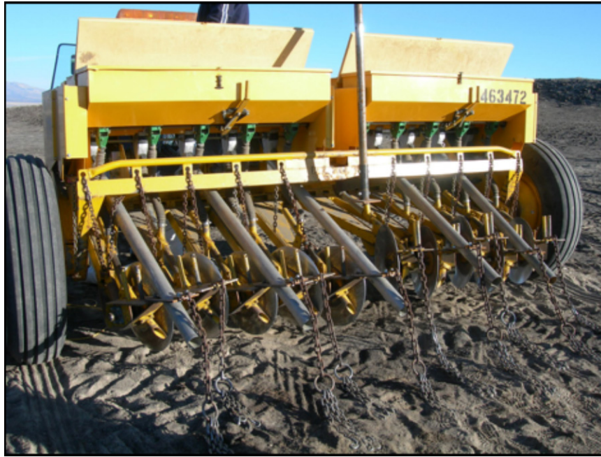
Figure 1. Rangeland drill (P & F Services manufacturer, Kemmerer model) modified to allow for different sizes of seeds in alternate rows. Note triple seed boxes and aluminum pipes installed to dispense seed from small seeds onto soil surface. On rows designated for small seeds, disks are raised above ground level to preclude furrow formation.
