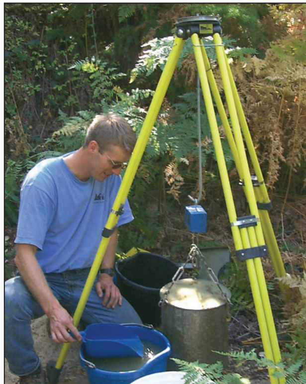
Figure 10 —Measure the sediment using a fiberglass survey tripod fitted with 100 lb (45 kg) capacity load cell.
