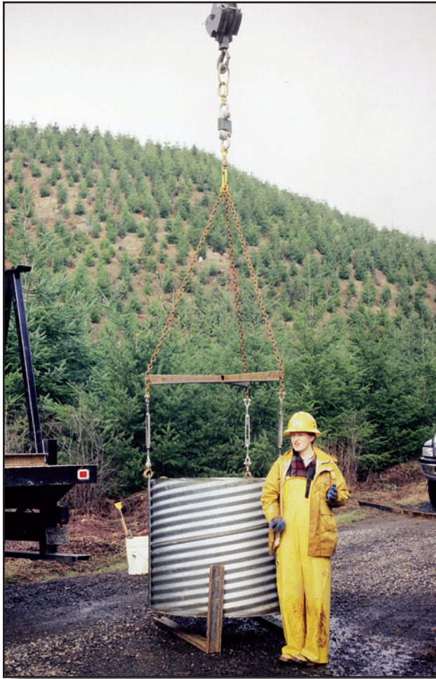
Figure 14 —A sediment collection tank is suspended from a crane by a radio-linked load cell. Notice the load distribution frame, turnbuckles used to level the water surface, and steel tipping bars below the tank.
