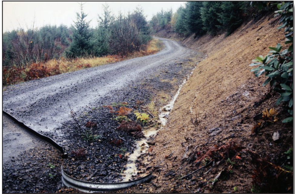
Figure 5 —A road runoff plot with ditch diversion inlet (in foreground) for the collection of runoff into the pipe.
