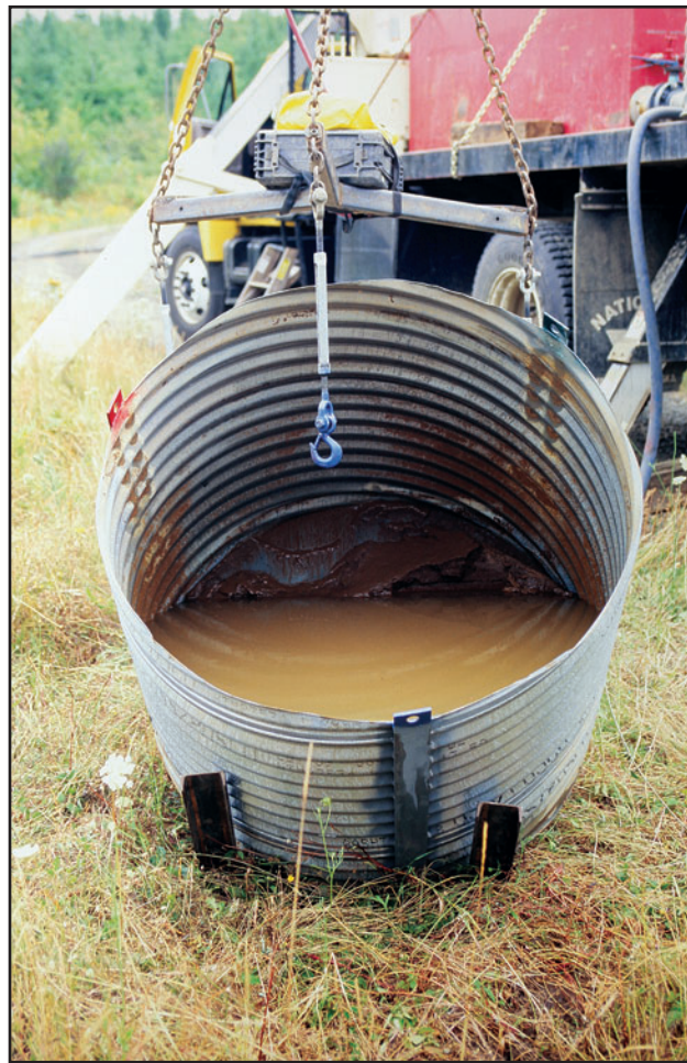
Figure 16 —A sediment tank is tipped over for sediment sampling. Note the L-shaped bars that support the tank during the sampling.
