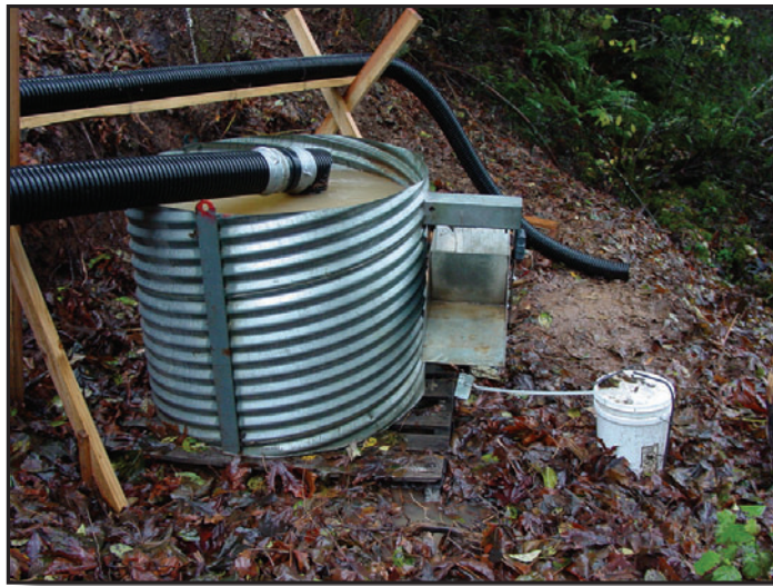
Figure 17 —A 20 gpm (76 lpm) tipping bucket and flow splitter in operation.
