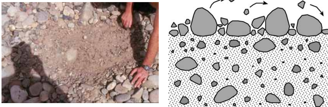
Figure 1. Distinction between the bed surface layer (armor) and the substrate, as commonly found in gravel-bed streams and rivers.
