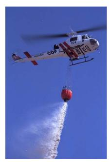
Helicopter buckets and fixed tanks can be equipped with foam injection systems. These systems inject foam concentrate into the water at a desired volume.
