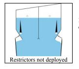
Flow restrictors are physical barriers inside the tank that can be deployed as needed. Restrictors decrease the opening area of the gate, slowing the rate of liquid exiting the tank.
